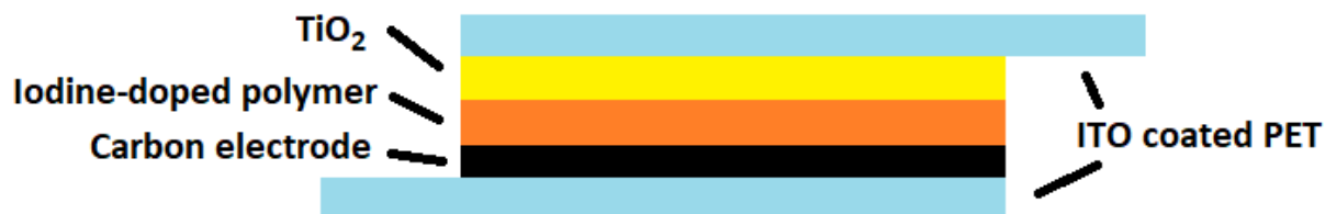
Figure 0.3: Cross sectional view of a completed solar cell.
