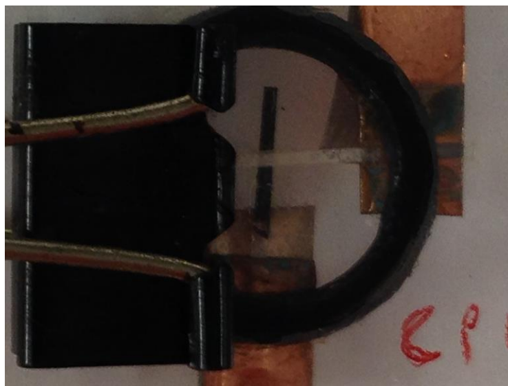
Figure 0.3: A fabricated photovoltaic cell sealed between two glass slides using a rubber O-ring.
