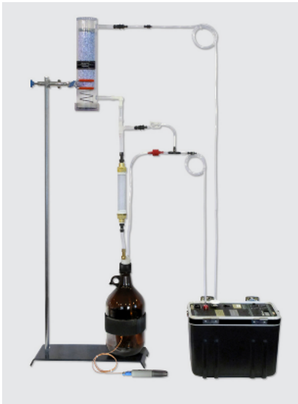
Figure 4-6. The DurrIDGE RAD7 “Big Bottle System” (DurrIDGE.com).
