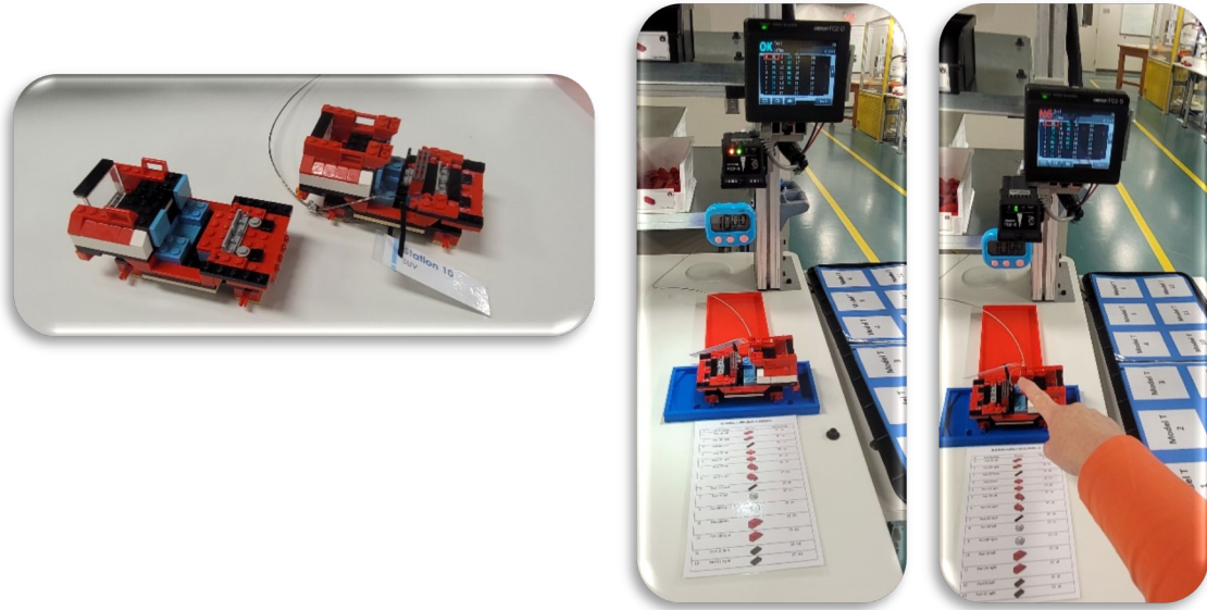
Figure 36: Quality Motivation and Performance Motivation Investigation: Treatments – Lean tool check piece (left), Industry 4.0 technology vision inspection camera (middle and right)
