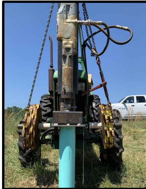
Figure 2. Tractor mounted hydraulic device is used to collect the soil cores.
