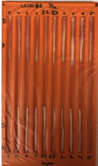
Figure 23: 3D printed tray with donor tendon sample placement
