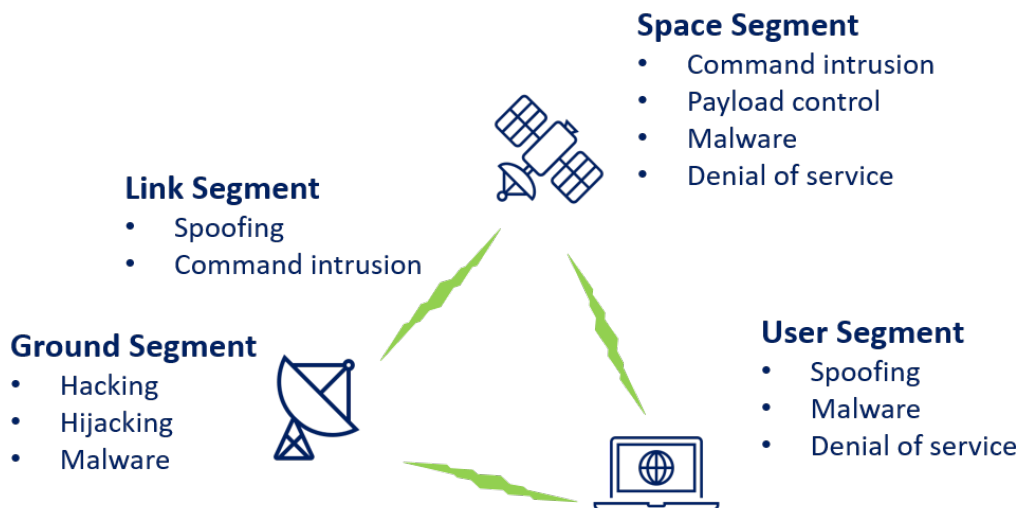
Figure 4.1: General overview of a satellite constellation infrastructure (ground, space, user and link segments) in association with potential threats.
