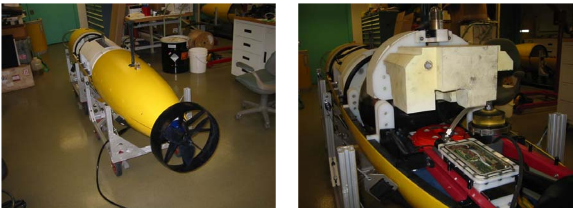
Figure 1.2: Example of an autonomous underwater vehicle with syntactic foam structural and buoyancy applications
