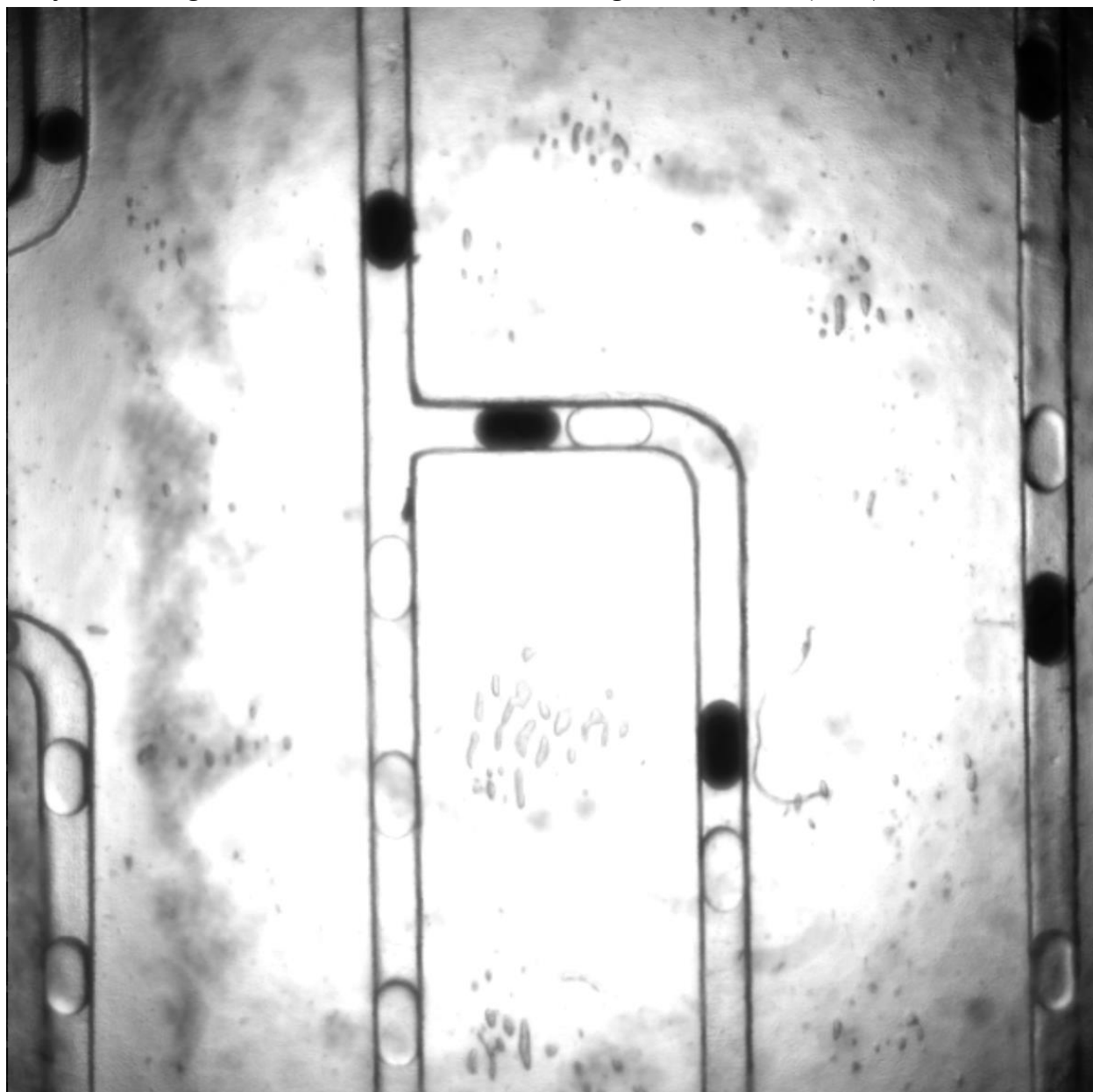
Figure 5.10 Control of two aqueous and one oil valve for alternating sample/reference flow using closed-loop automation
