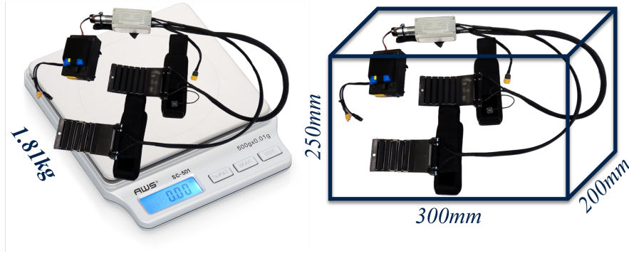
Figure 4.13: Size and weight measurements for CASET. Size measurements took into particular consideration CASET’s transportability, so the smallest box the entire device could reasonably fit into was measured.
