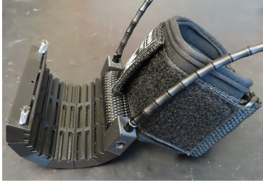
Figure 4.6: The first working CASET gripper. This version was large to overcompensate for the force requirements and included slits for straps to run through.
