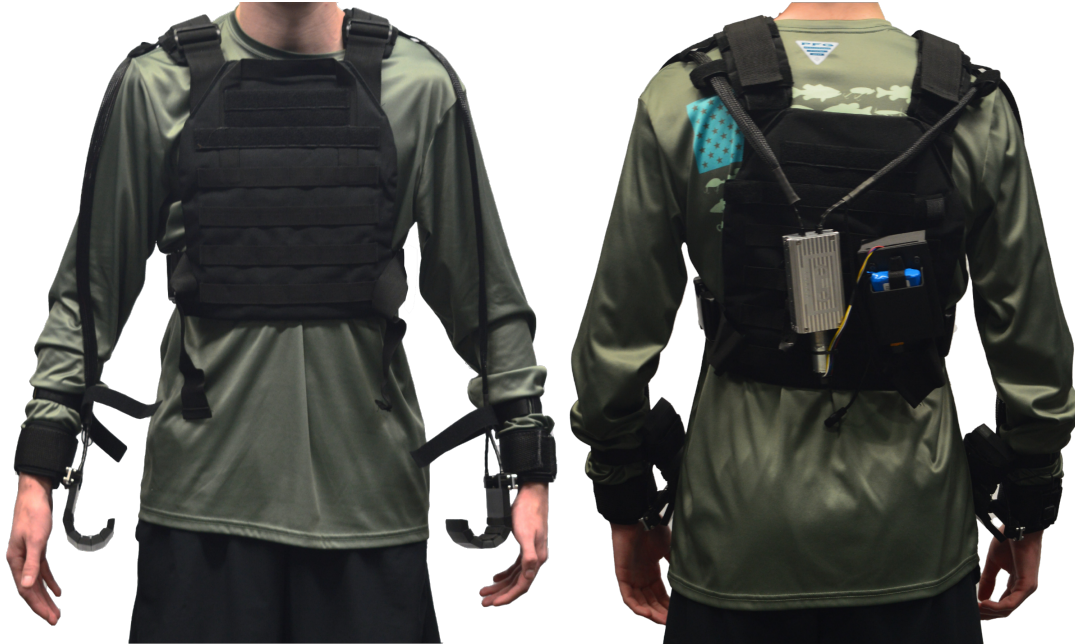
Figure 4.9: The Curling Artificial Soft Exoskeleton (CASET). CASET is a lift-assistance device that offloads carry weight from the fingers to the wrist to increase carry time and reduce fatigue. Front (left) and rear (right) views shown in the enabled and disabled states respectively.
