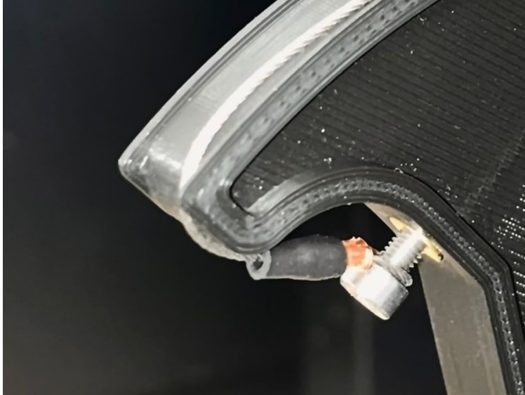
Figure 5.2: A close up of the cable tensioning system for a single SER capstan. tightening the screw increases tension of the cable which allows for adjustability and easy compensation for cable stretch.
