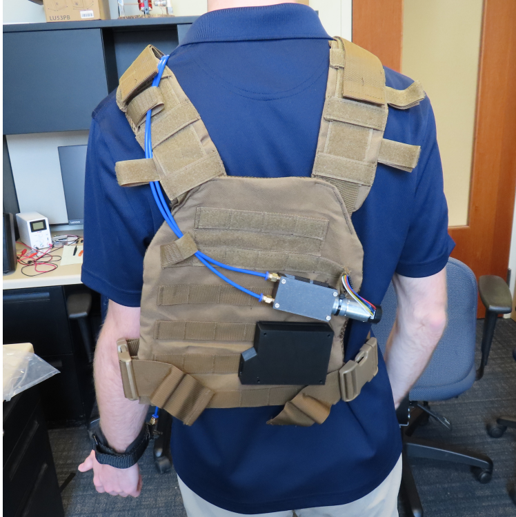
Figure 4.4: Overview of the second working CASET prototype. This version could hold 10-20lbs dumbbells, but when weight was increased any more the 3D printed parts would fail under loading.
