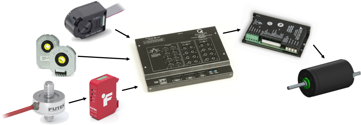
Figure 3.12: Input/output flow with the Quanser Q8 system and all SER components. Encoders and the load cell provide all inputs and the Q8 running SIMULINK produces voltage outputs to the DC motor controllers.
