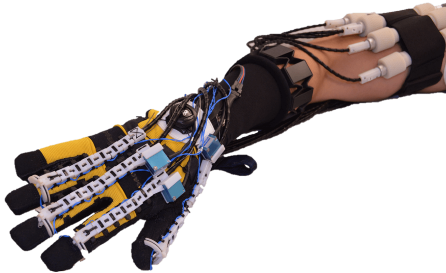
Figure 2.6: The SeptaPose Assistive and Rehabilitative (SPAR) glove developed by Rose. This wearable device uses cables and 3D-printed links to provide grip assistance while using EMG to detect user intent.
