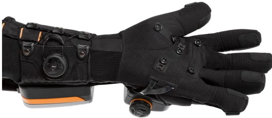
Figure 3.2: A single HaptX G1 glove. The gloves come in four different sizes, and all work off the same HaptX air pack system to provide tactile feedback at the fingertips and force feedback to finger flexion.
