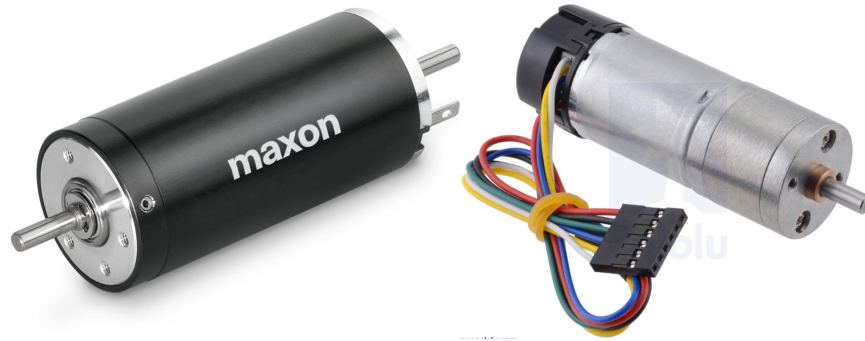
Figure 2.13: The (left) Maxon 20W RE25 [5] and (right) Pololu 8.4W with 75:1 gearbox [6] DC motors used in SER and CASET respectively. In this case, the higher cost of the Maxon motor results in better efficiency and responsiveness, and access to Maxon’s own 4096 CPR encoders. For CASET, a cheaper motor with a build in gearbox and less accurate encoder was desired.
