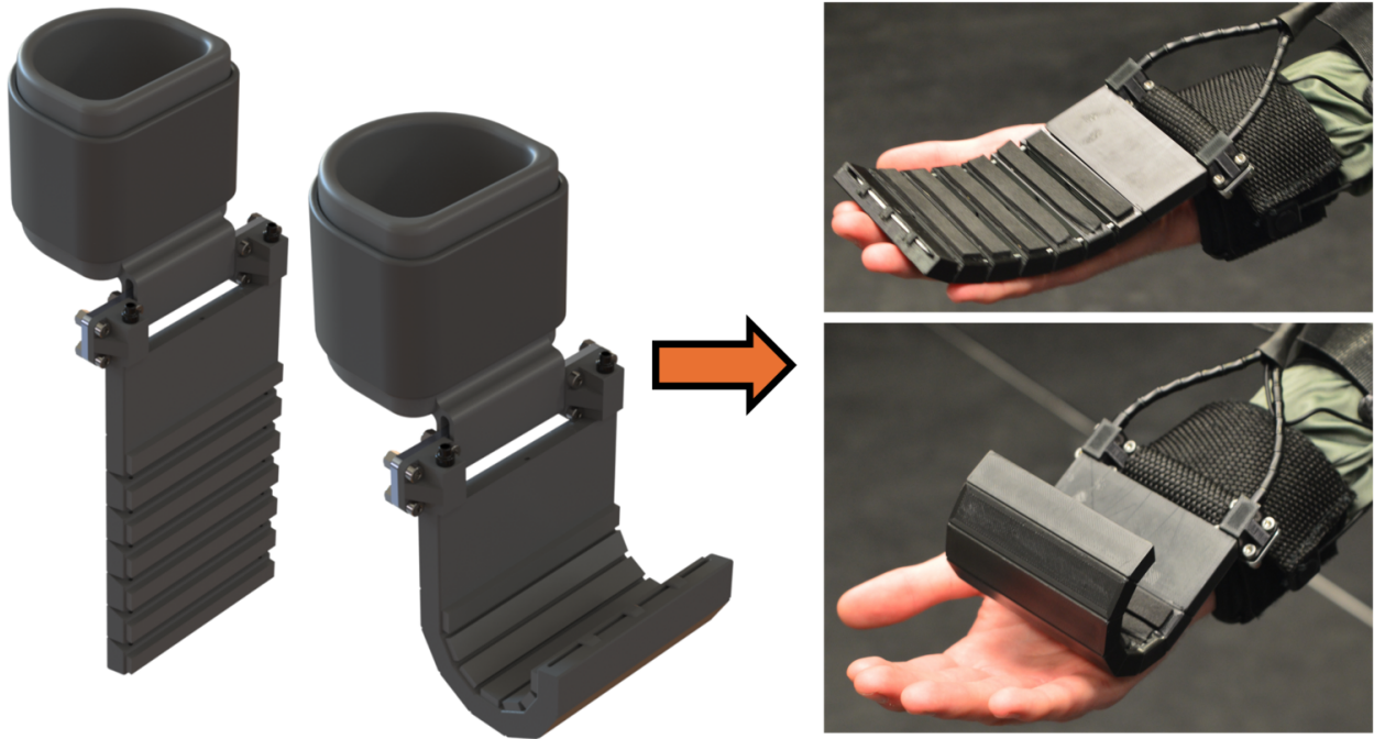
Figure 4.11: The CASET grippers, in CAD and reality. The SPAR-inspired working principle can be seen in action through the curling motion when tension is applied.
