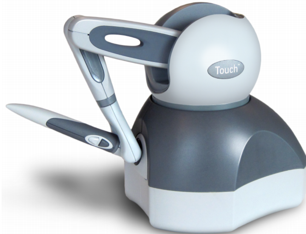
Figure 2.4: The Touch haptic device produced by 3D Systems [1]. This PHANToM Premium inspired grounded kinesthetic robot is used in various haptics experiments and drawing/training programs.
