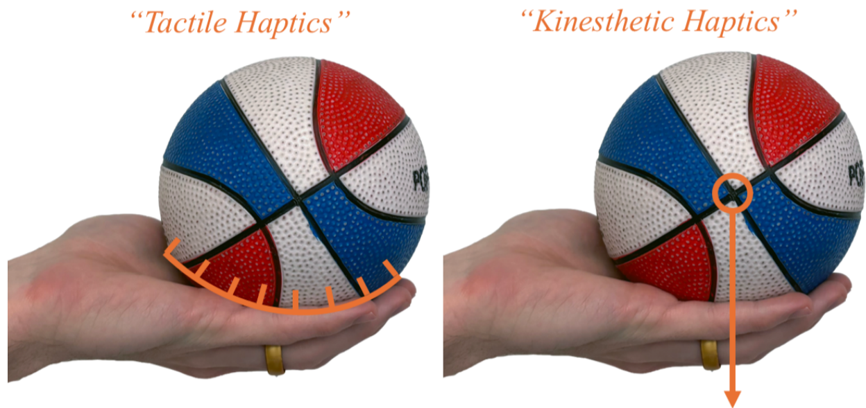
Figure 2.1: A user holding a textured ball, with the texture or inertia of the ball interacting with the user shown. The ball’s inertia is best simulated virtually using kinesthetic haptics, whereas the texture and general ‘feel’ of the ball is best simulated using tactile haptics.
