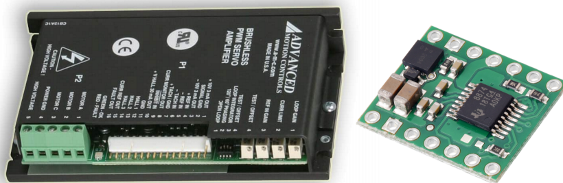
Figure 2.14: The (left) AMC CB12A1C [7] and (right) Pololu DRV8874 DC motor [8] drivers used in SER and CASET respectively.
