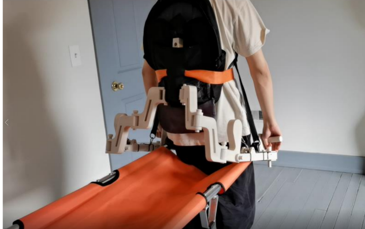
Figure 2.8: A supernumerary device developed by Liu et al. to offload litter carry, similar to the CASET device in this manuscript.
