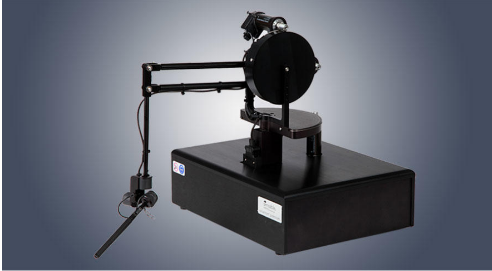
Figure 2.3: The PHANToM Premium haptic device. This early kinesthetic robot provided the foundation for many capstan-driven, multi-DOF, force-feedback kinesthetic robots that came after it such as the 3D Systems Touch and SER.
