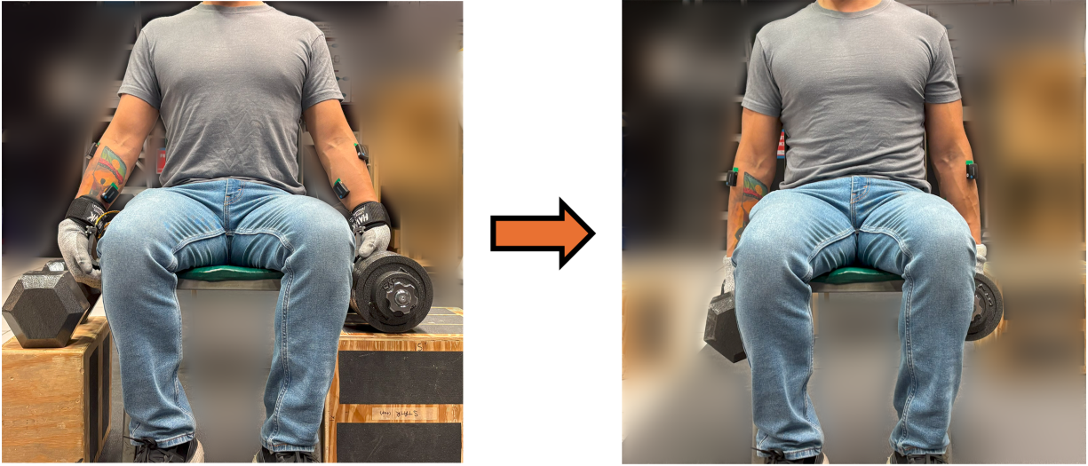
Figure 4.15: User interaction before and after holding weights with CASET. After the participant begins by lifting the weights slightly, testers pull the weight stands away and replace them with foam pads for the participant to release the weights upon.
