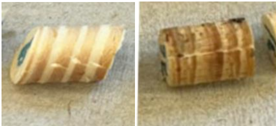
Figure 2. The slanted core segment (left) and the normal core segment (right) of 5 rings of longleaf pine.
