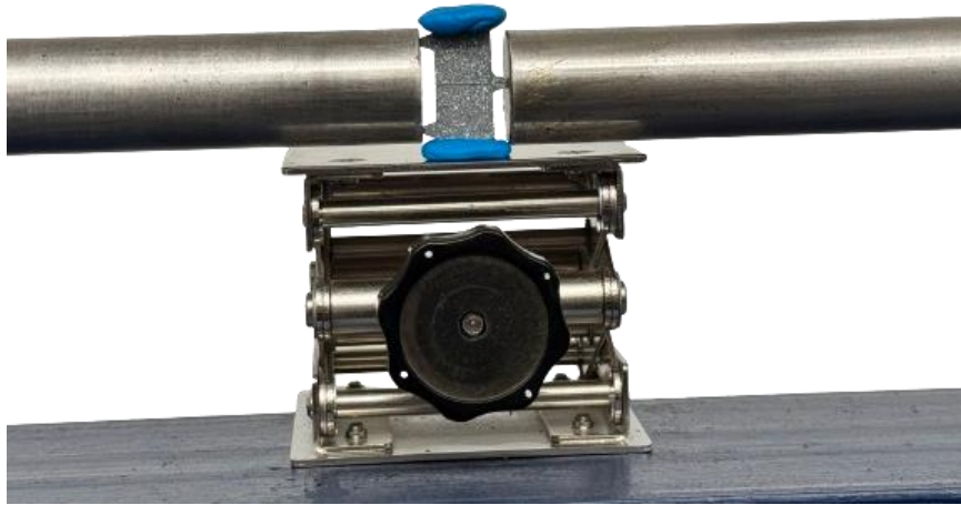
Figure 4.7: Specimen held in place between the incident and transmitted bars with putty and support table
