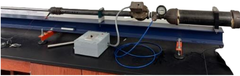
Figure 4.5: Photograph of the gas-gun apparatus aligned with the incident bar of SHPB
