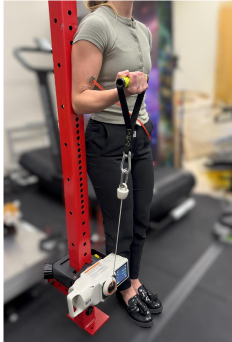
Figure 4.2: The participants performed standing bicep curls with the non-dominant arm while the BeyondPower Voltra unit (mounted at the base of the rack) supplies cable resistance through a D-handle. The upper arm is braced against the rack to minimize shoulder motion, ensuring that elbow flexors do the primary work. An ADXL367 accelerometer secured to the bicep records MMG, and the Voltra's onboard sensors track force and kinematics for every repetition.
