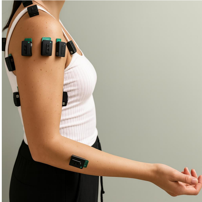
Figure 1.4: Multi-electrode surface EMG setup for upper limb muscle analysis. Low profile wireless sensors are placed over the muscle bellies to capture muscle activity while allowing unrestricted movement. Figure reproduced from [5].
