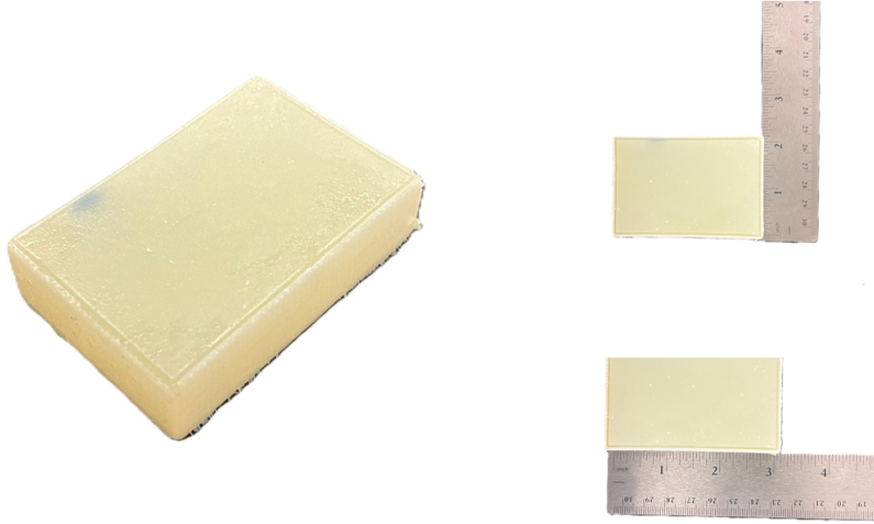
Figure 3.8: Rectangular prism ultrasound test coupons printed with varying J5 DAP material formulations. These samples were used to assess the acoustic properties and echogenicity of different material combinations under ultrasound imaging.
