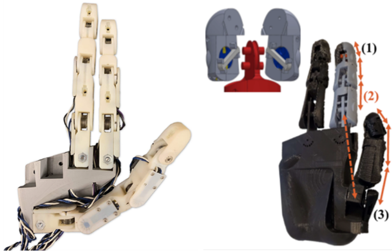
(b) Yousaf et al. used an anthropometric model with steel springs for compliance. Hall effect sensors provide frictionless position sensing and a joint interaction. (figure reproduced from [51]) (c) Baskaran et al. produced 3D-printed anthropomorphic hand with a potentiometer for position sensing and a rubber-pulley system for joint compliance
