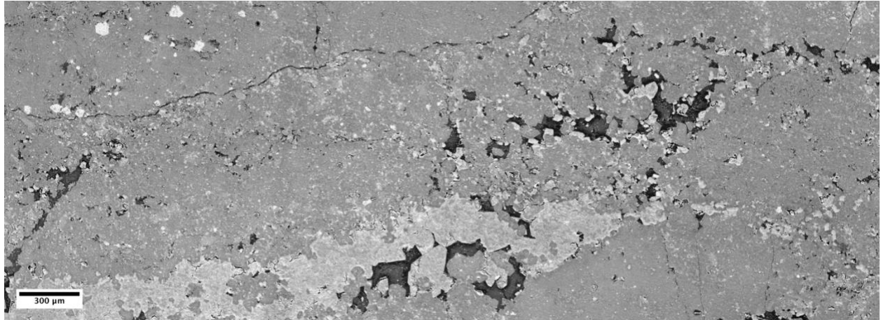
Figure 2.2. SEM BSE image of the sample thin section from Cassville Well 1.
