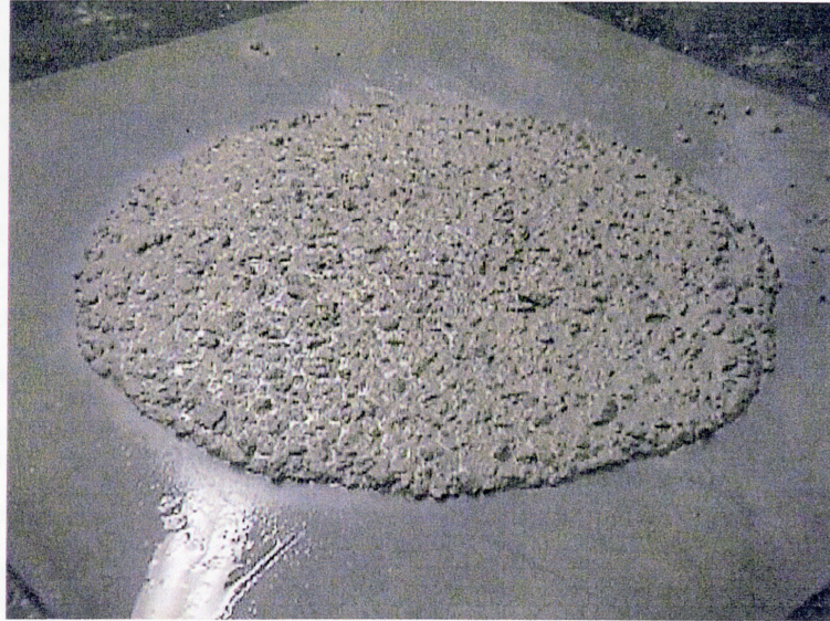
Figure 2-3: Typical visual stability index rating of 0 (PCI 2003)
