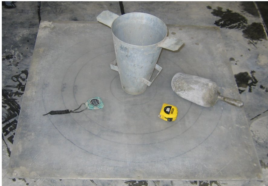
Figure 3-3: Testing equipment for slump flow test
