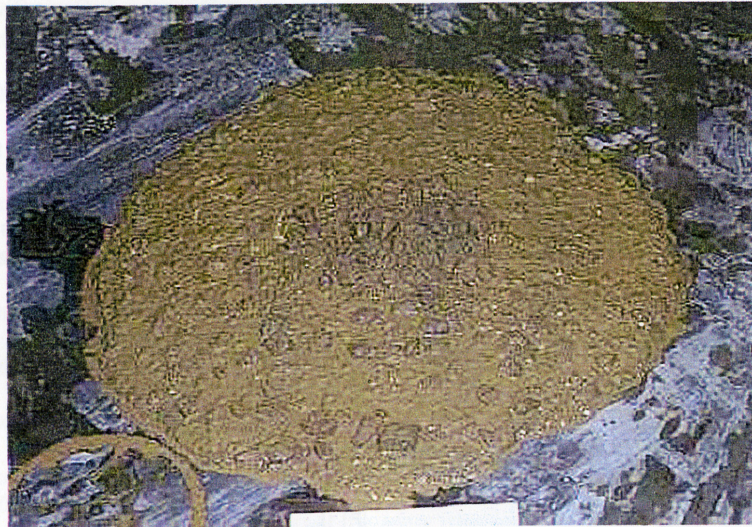
Figure 2-10: Typical visual stability index rating of 3 (PCI 2003)
