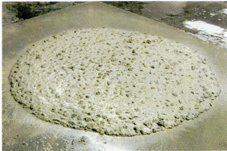
Figure 2-4: Typical visual stability index rating of 0.5 (PCI 2003)
