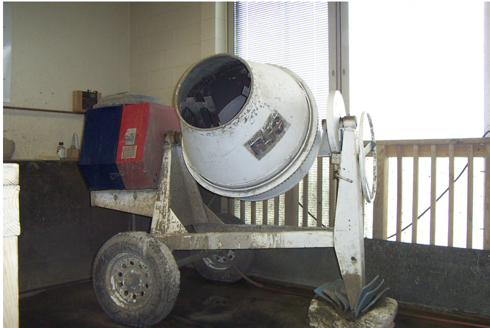
Figure 3-2: 12-ft 3 concrete mixer used for this project
