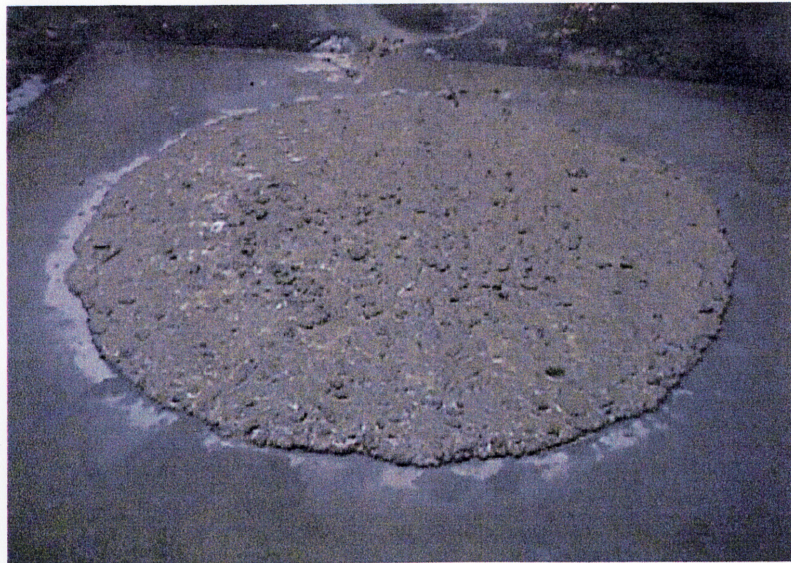
Figure 2-6: Typical visual stability index rating of 1.0 (PCI 2003)
