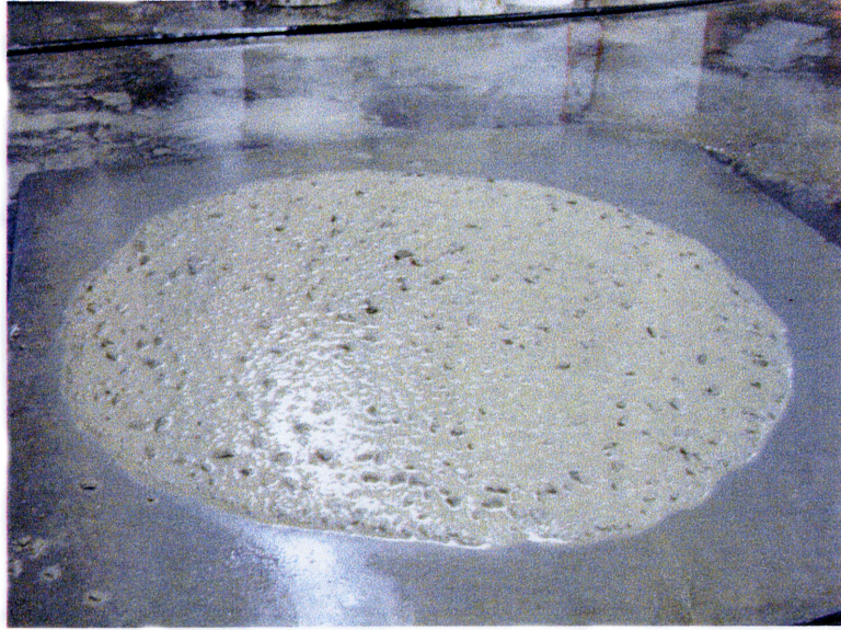
Figure 2-9: Typical visual stability index rating of 2.0 (PCI 2003)
