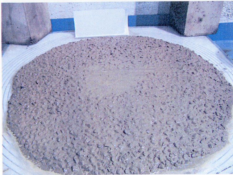
Figure 2-8: Typical visual stability index rating of 2.0 (PCI 2003)
