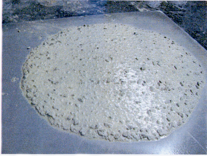
Figure 2-7: Typical visual stability index rating of 1.5 (PCI 2003)
