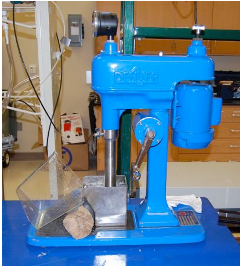
Figure 3-20: Denver D-12 Flotation Cell.
