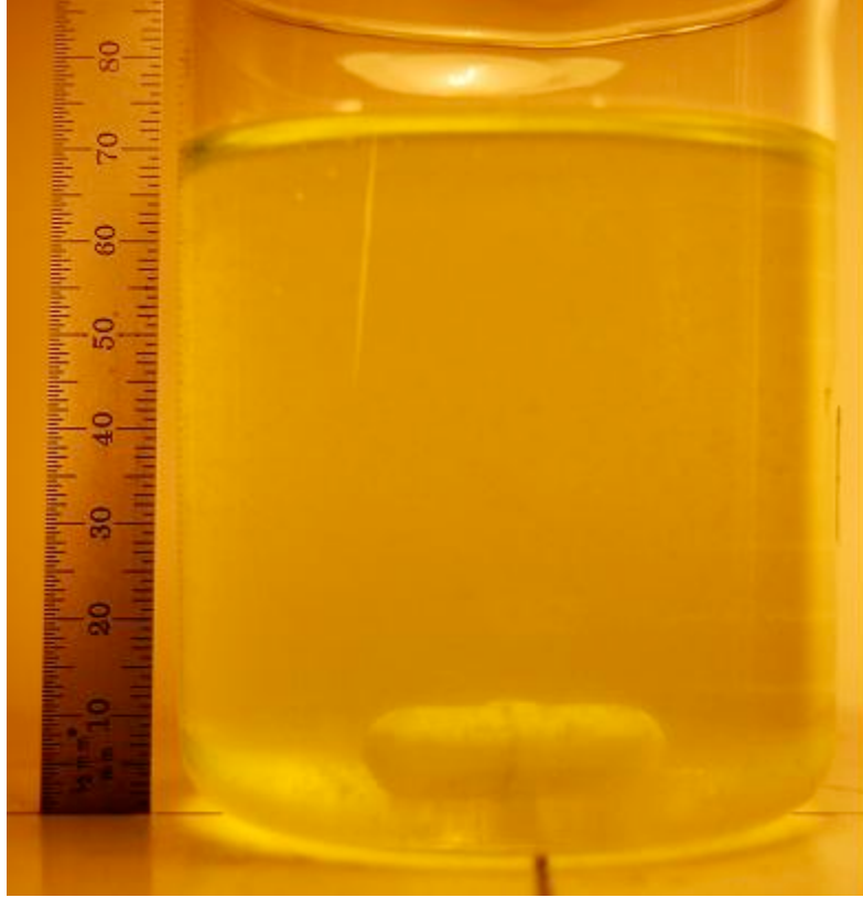
Figure 3-5: Typical flocculation beaker test 1 minute after addition of secondary flocculant. Corresponds to iron nitrate and chitosan concentrations of 50 ppm and 1.25 ppm respectively.
