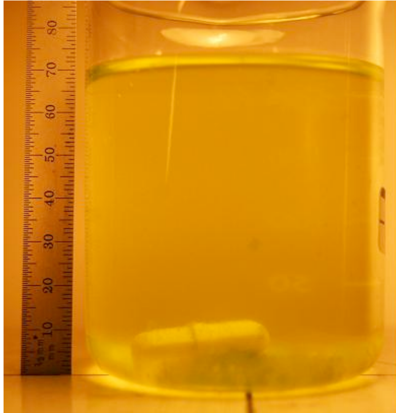
Figure 3-6: Typical flocculation beaker test after 15 minutes of settling. Corresponds to iron nitrate and chitosan concentrations of 50 ppm and 1.25 ppm respectively.
