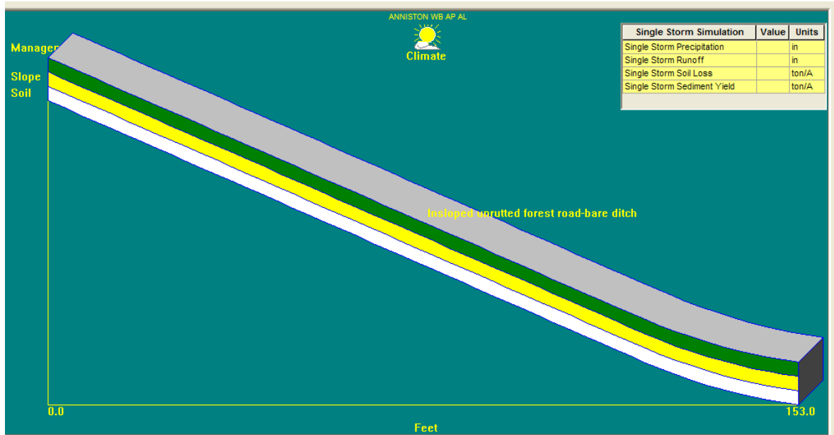
Figure 3.6 -- Steep slope with insloped unrutted forest road-bare ditch management layer.
