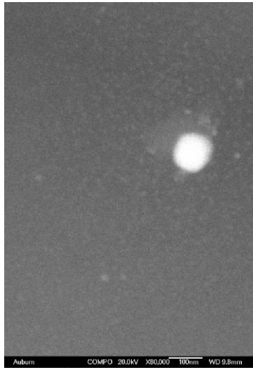
Figure 3.1. SEM image of 50 nm Ag nanoparticles
