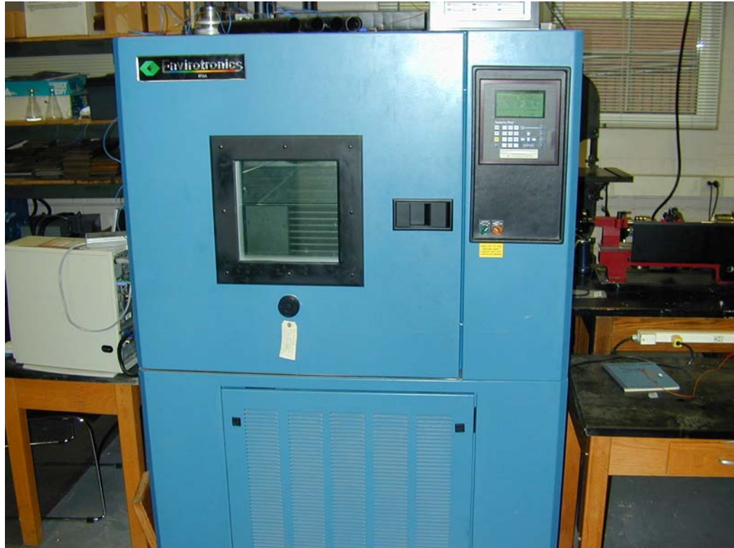
Figure 11.1.3. Environmental chamber used for temperature test
