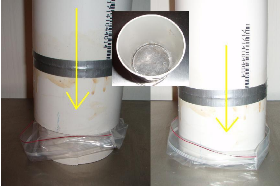
Figure 18B: Fumigation pot being slipped over basal fumigation ring and view through top of pot (Weed Experiment 8).
