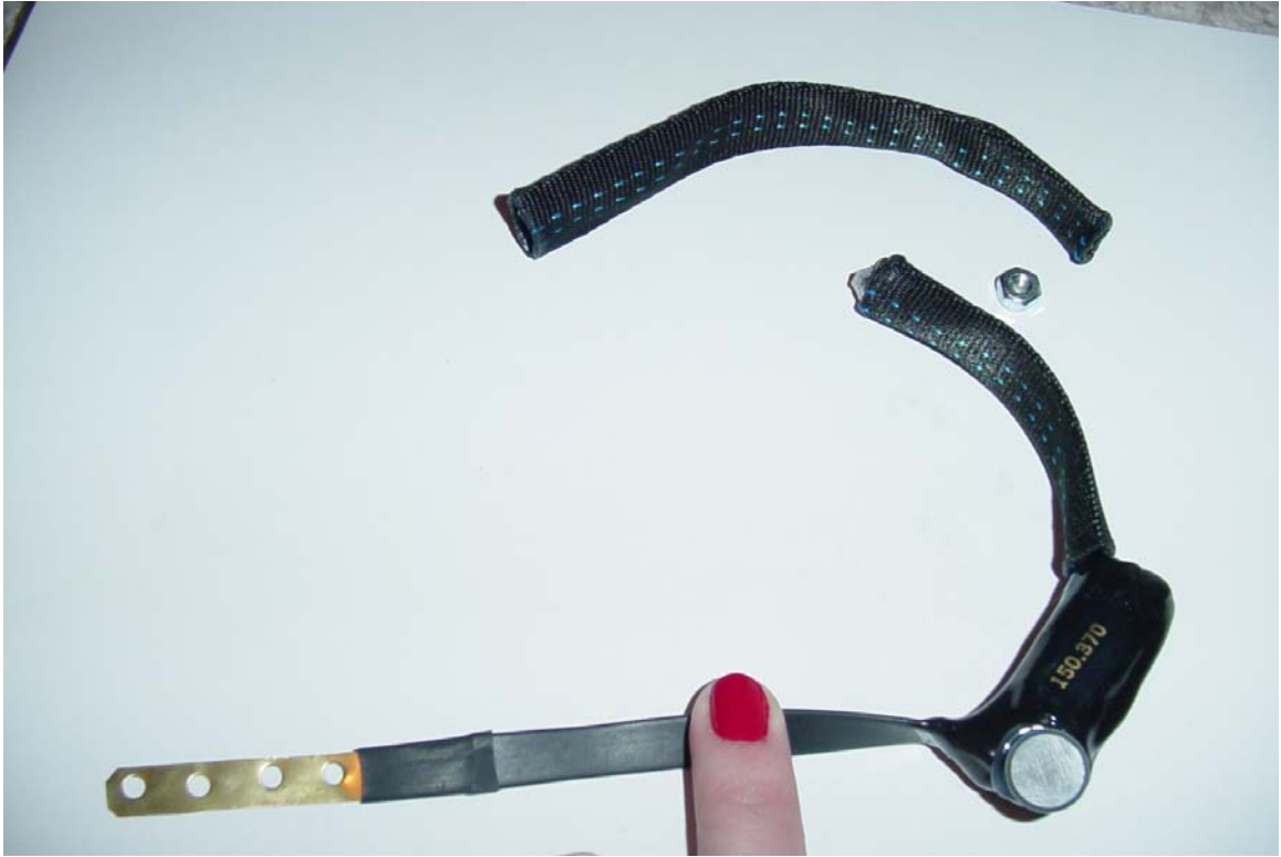
Figure 3. Feral Cat Radio Collar. Radio transmitter and adjustable metal collar with loop antenna used in feral cat home range and habitat use study in Auburn, Alabama 2003-2005.
