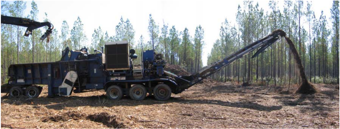
Fig. 1.7. Clean chip residual is processed in the field through a horizontal grinder before sale to a pulp mill as fuel.
