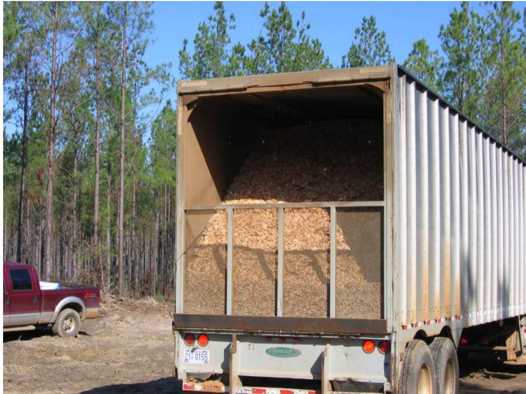
Fig. 1.4. 'Clean chips' loaded into a van for transport to a pulp mill.
