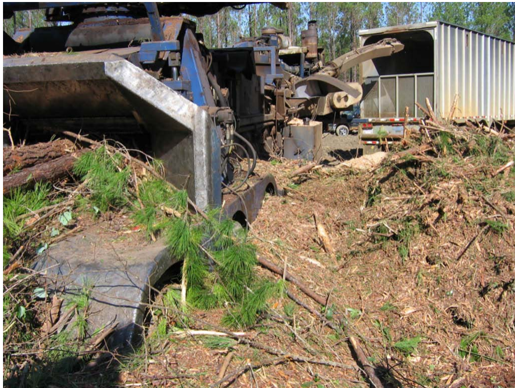
Fig. 1.2. Total tree harvesting machine. Trees are fed into a flail which de-limbs and debarks the trees before they are fed into a chipper which results in small, uniform 'clean chips' used for paper manufacturing. There is a less than 1% tolerance for the presence of pine bark in 'clean chips.'
