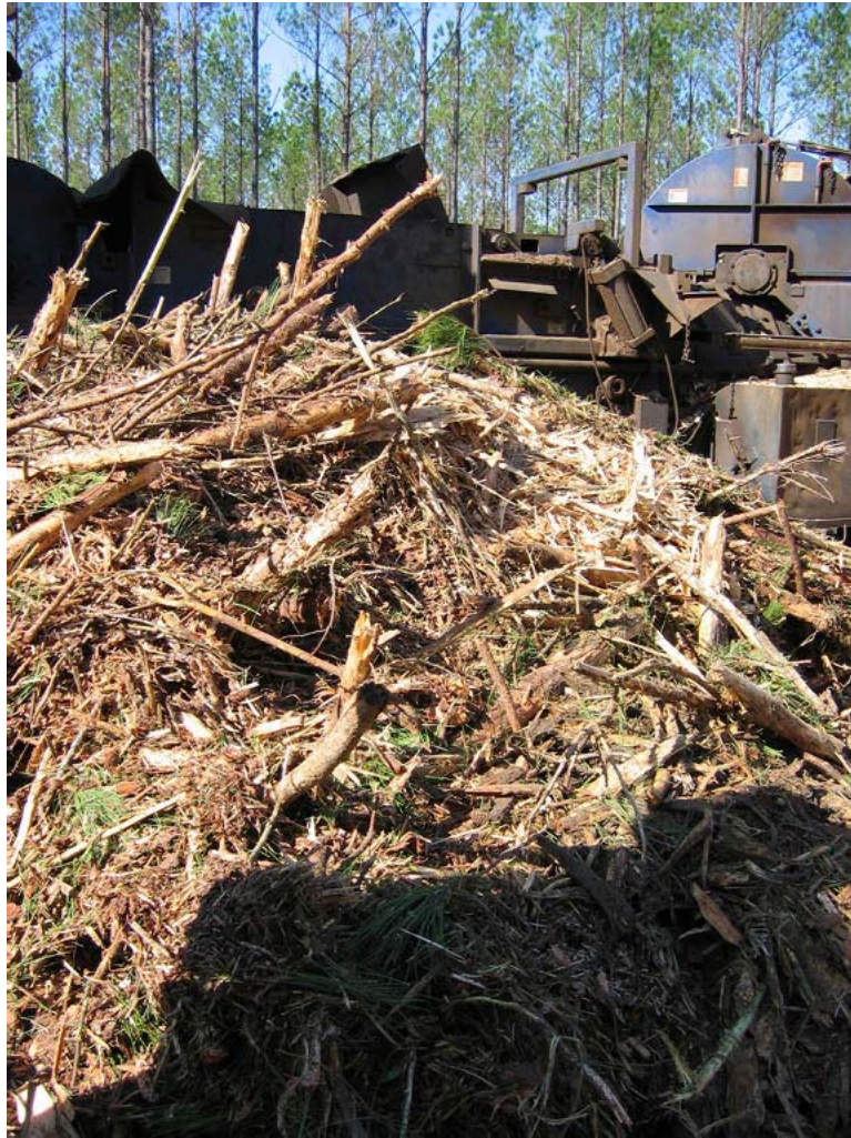
Fig. 1.5. Residual material resulting from in-field harvesting for 'clean chips.' This material is processed into clean chip residual.
