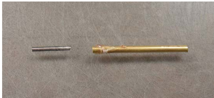
Figure 11.6.1 Photograph of the tool-hardened steel stub and brass tubing
