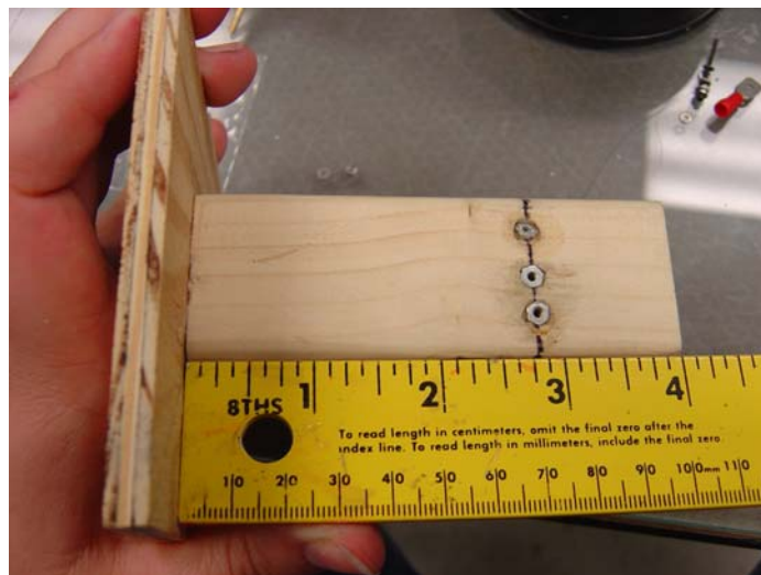
Figure 11.8.1 Base Assembly Before Ready for Tensioning Screws
