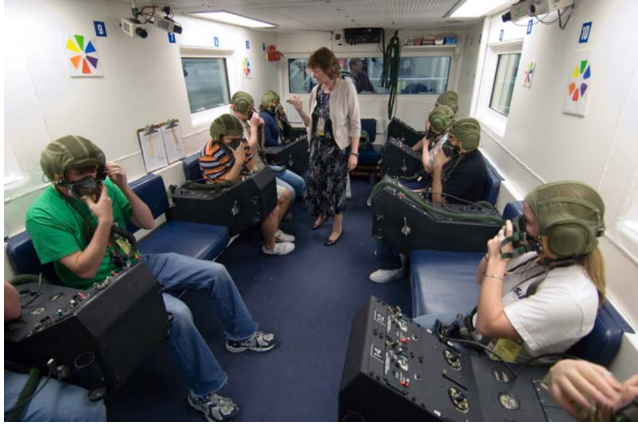
Figure E.5. Team Preflight Physiological Testing in Altitude Simulator
