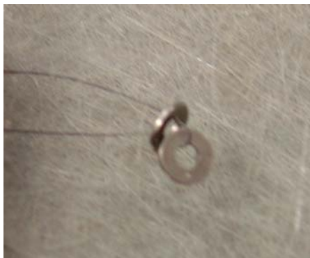
Figure 11.7.2 Photograph of SMA Loop and Washers Tightened
