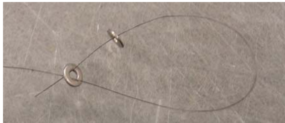
Figure 11.7.1 Photograph of SMA Loop with Washers for Anchoring
