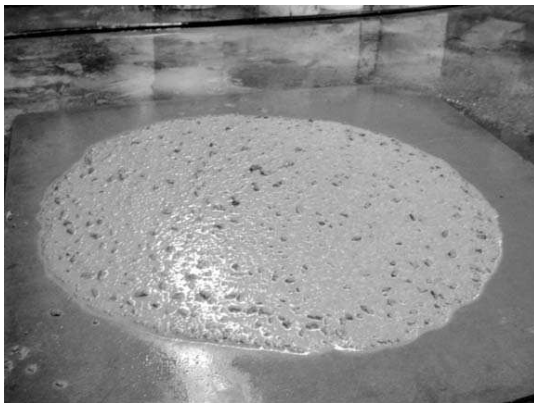
VSI = 2 – Evidence of a mortar halo and water sheen
