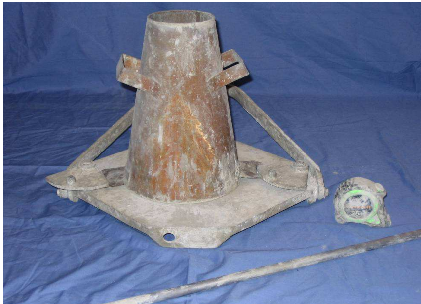
Figure 4.6: Water slump testing equipment and setup
