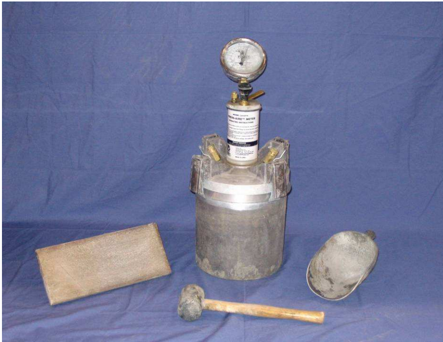
Figure 4.10: Air content and unit weight equipment
