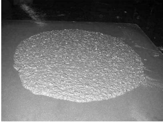
VSI = 0 – Concrete mass is homogeneous and no evidence of bleeding
