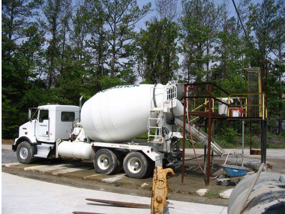
Figure 5.15: Concrete truck at wash station platform
