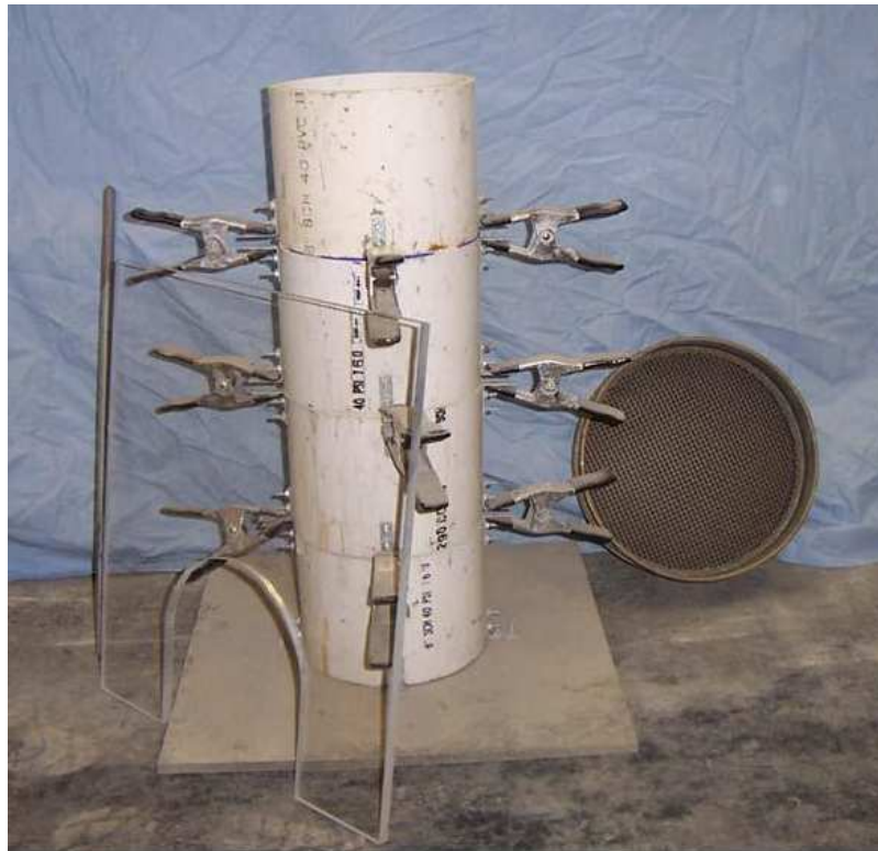
Figure 4.9: Segregation column equipment and setup (Bailey 2005)
