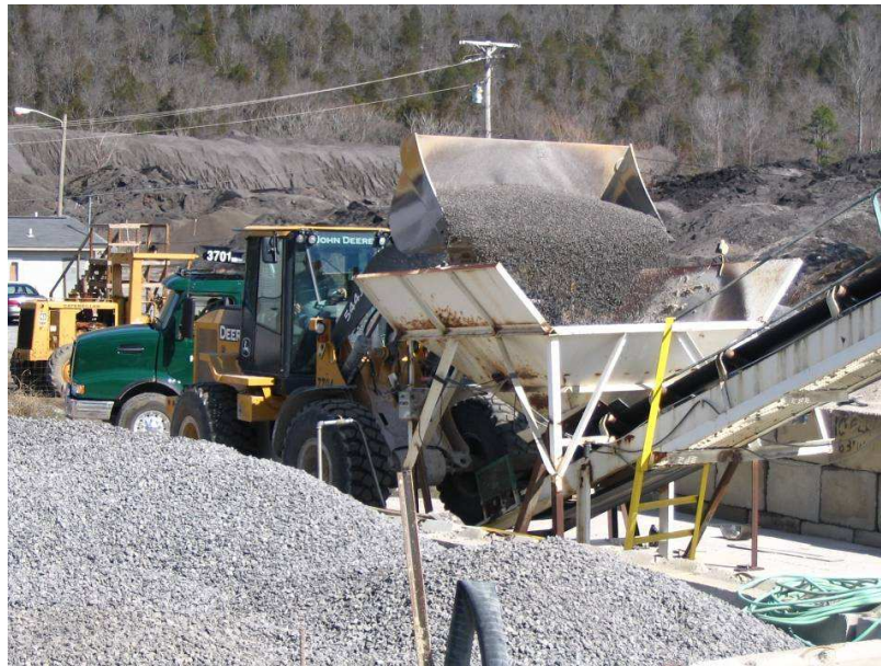
Figure 5.13: Loading aggregate from stockpile
