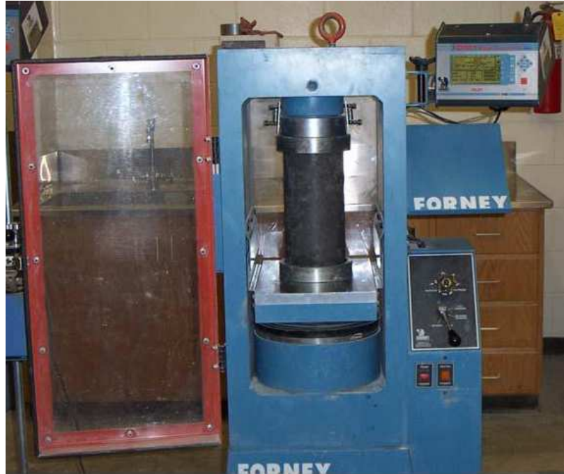
Figure 4.12: 600-kip Forney compression machine (Bailey 2005)
