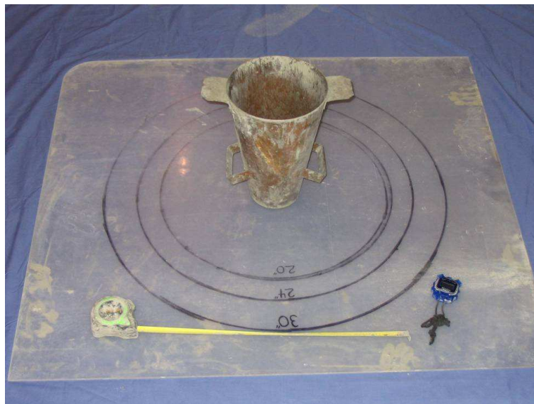
Figure 4.7: Slump flow testing equipment and setup
