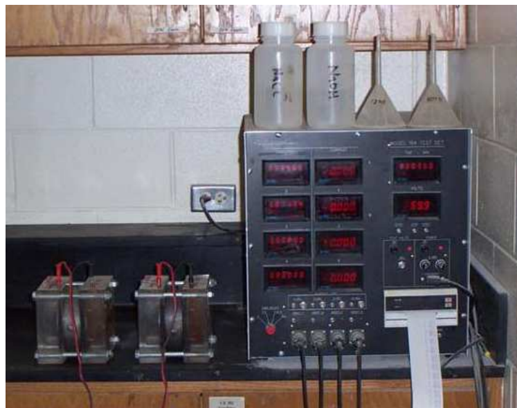
Figure 4.15: Model 164 test set and Proove' It cells (Bailey 2005)
