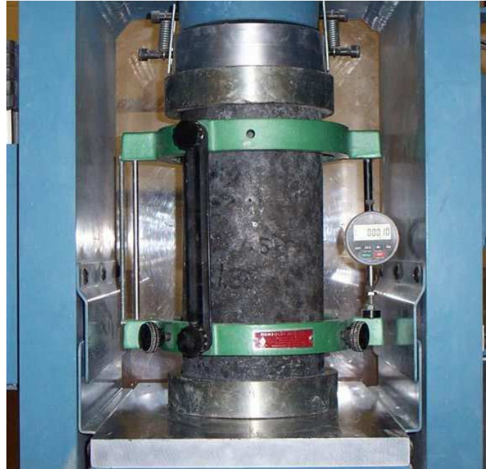
Figure 4.13: Concrete cylinder with compressometer attached (Bailey 2005)
