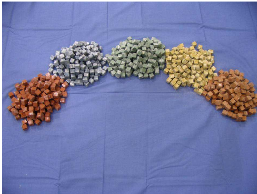
Figure 4.5: Colored 1/2 in. mortar cubes
