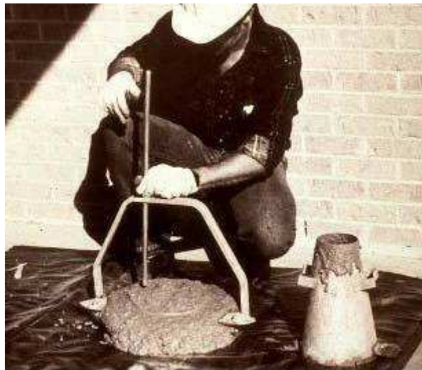
Figure 2.21: Concrete with proper workability and mixture design for tremie placement (O'Neill and Reese 1999)
