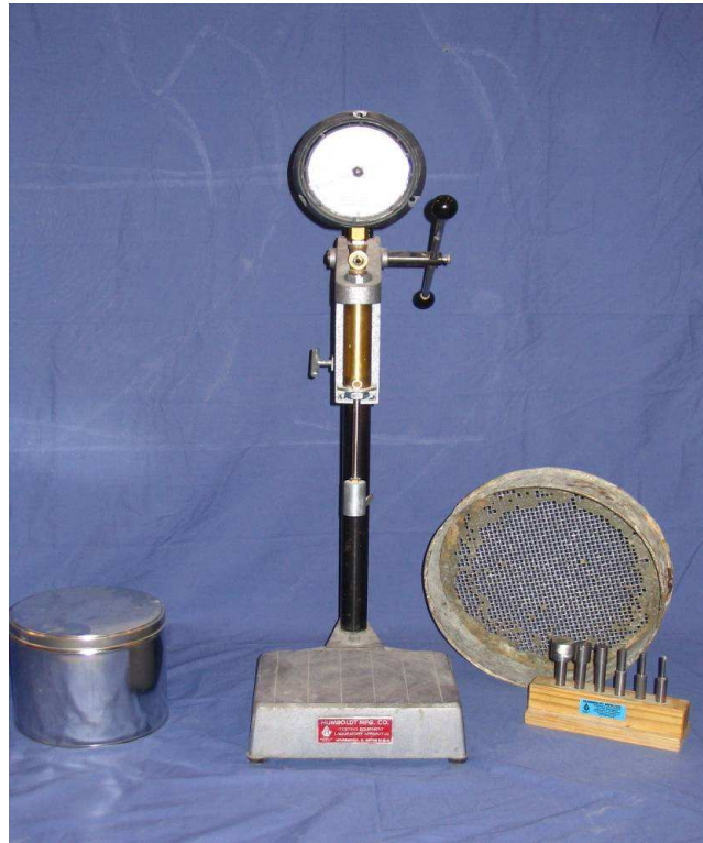
Figure 4.11: Setting test equipment
