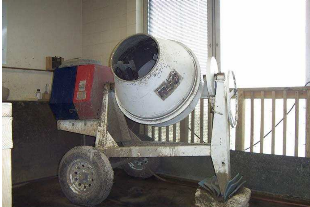
Figure 4.2: 12-ft 3 concrete mixer (Bailey 2005)
