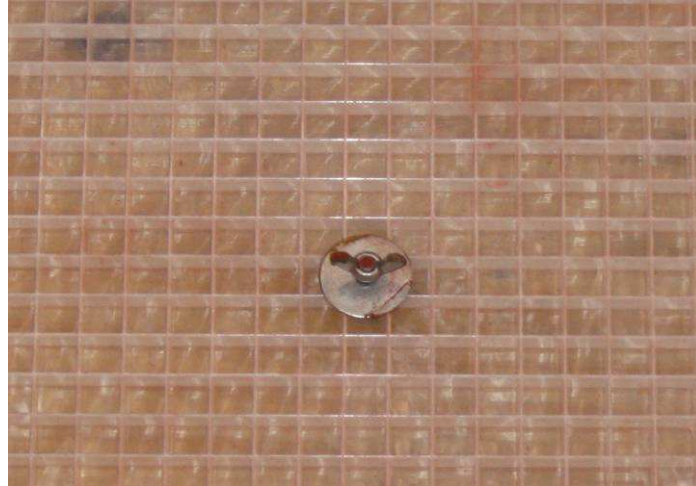
Figure 4.4: Screw, washer and wing nut configuration used to anchor mortar cube form
