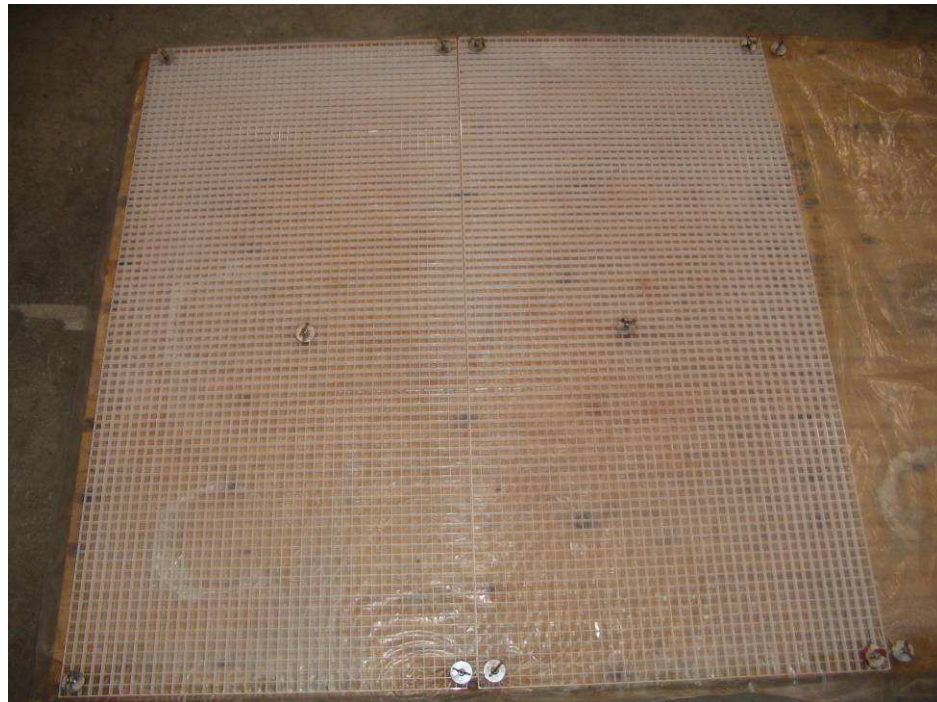
Figure 4.3: Polystyrene light diffuser panel used for mortar cube form
