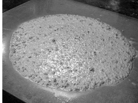
VSI = 1 – Concrete shows slight bleeding observed as a sheen on the surface
