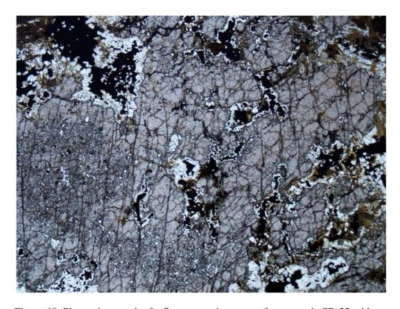
Figure 68: Photomicrograph of a first generation garnet from sample SR-22 with two fracture sets. The dominant fracture set is oriented roughly vertical in this photo. The subordinate set is oriented roughly 50 °Clockwise from vertical. Inclusions are opaques with plagioclase rims. Plane-polarized light. Horizontal FOV = 5.5 mm.
