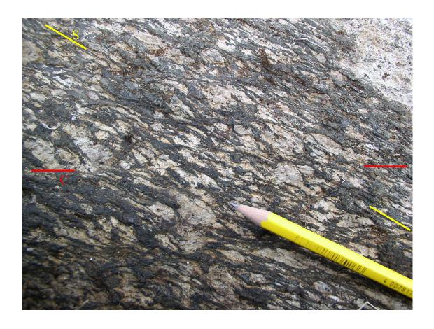
Figure 36: Photograph of paired S-C fabrics in the eclogitized shoulder of shear zone II. View is vertical. S-plane – yellow. C-plane – red.
