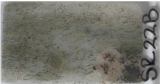
Figure 66: Scans of two thin sections from Storvatnet sample SR-22. Foliation was not clear, therefore, these two thin sections were cut perpendicular to each other and parallel to elongation lineation. Plastic flow structure wraps around undeformed, but retrograded garnet. The flow structure is defined predominantly by the fine grained, dynamically recrystallized plagioclase. Short dimension of slide is 2 cm.
