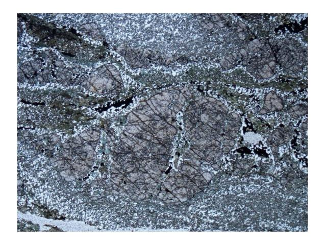
Figure 52: Photomicrograph of one well-developed and one poorly developed fracture set in a relict  $1^{\text{st}}$  generation garnet with no rim from sample NFA-17. The dominant fracture set is inclined moderately to the right; the subordinate set is inclined shallowly to the left. Plane-polarized light. Horizontal FOV = 5.5 mm.
