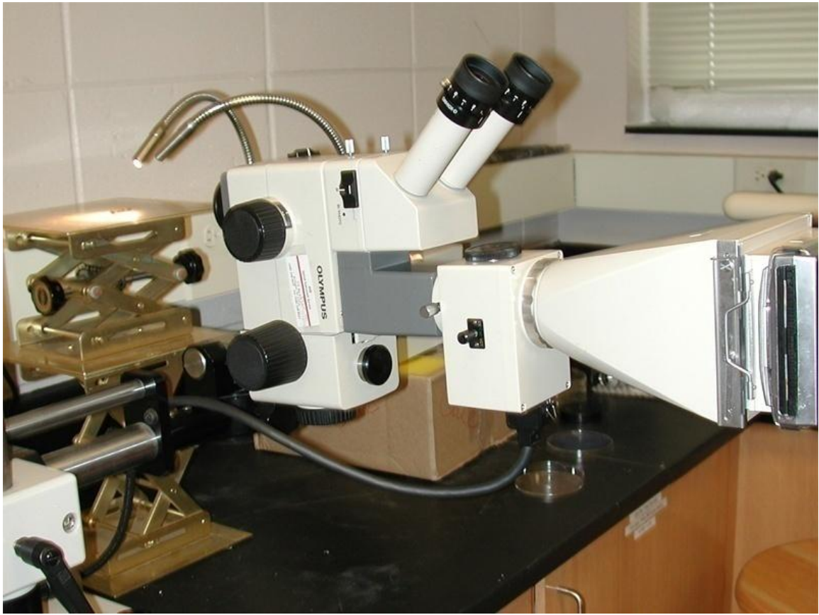
Figure 3–Stereo-light microscope setup oriented to permit a side view of the inoculum droplet.
