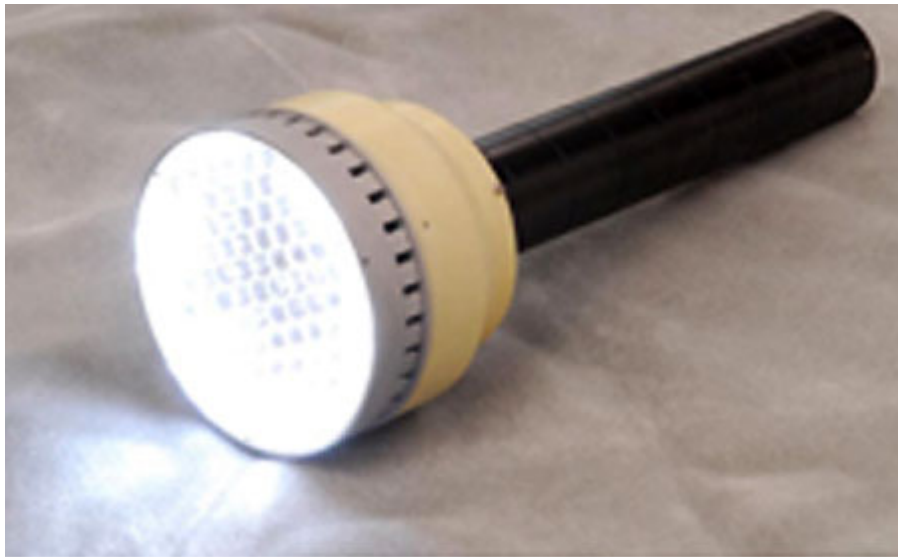
Figure 2.4: Prototype light-emitting diode incapacitator [25]
