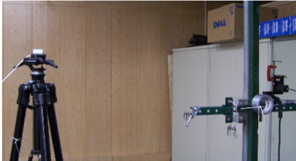
Figure 3.14: Experimental Setup for long range calibration. Note that the camera is separated from the pan/tilt device.
