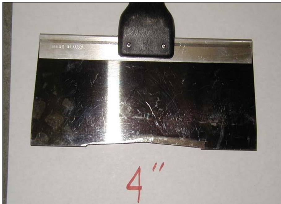
Figure 4.8: Modified 4-inch V-notched Trowel
