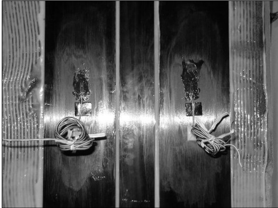
Figure 5.4: Typical Strain Gauge Installation to FRP Surface for Exterior Girder
