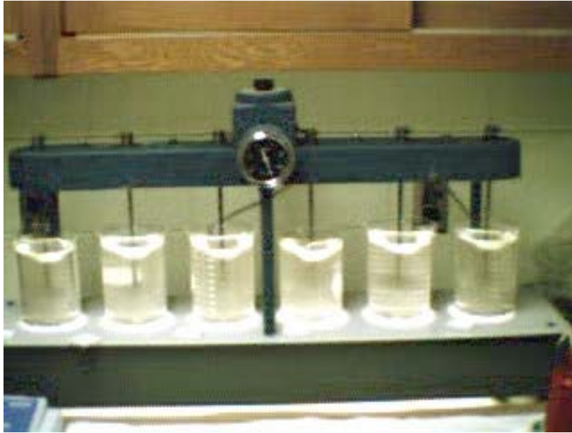
Figure 4.0. Jar Test apparatus mixing at 100 rpms with \text{FeCl}_2 Coagulant.
