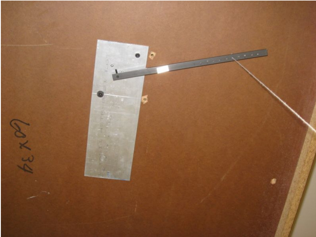
Figure 5.3: Bottom view of the Setup with Aluminum Beam (Tow Link) and Thread (Tether)
