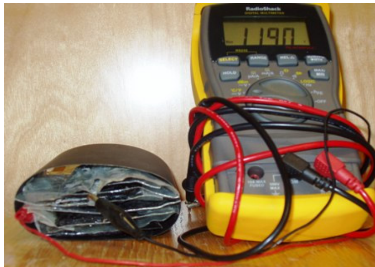
Figure 4.5 A stack of 10 batteries connected in series
