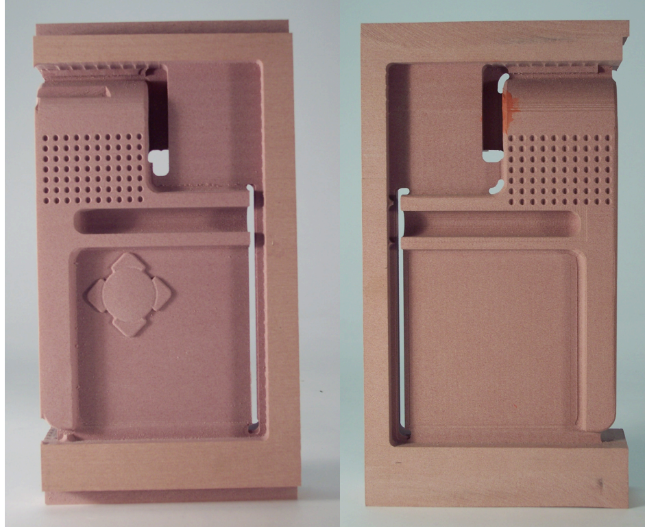
Figure 7. The parts were milled using RenShape 450 on a Roland CNC Router
