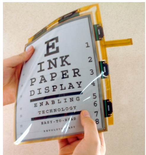
Figure 4. e-ink technology for displays
