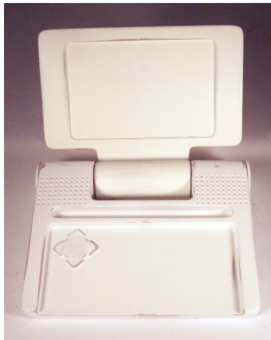
Figure 10. The model was sanded and primed
