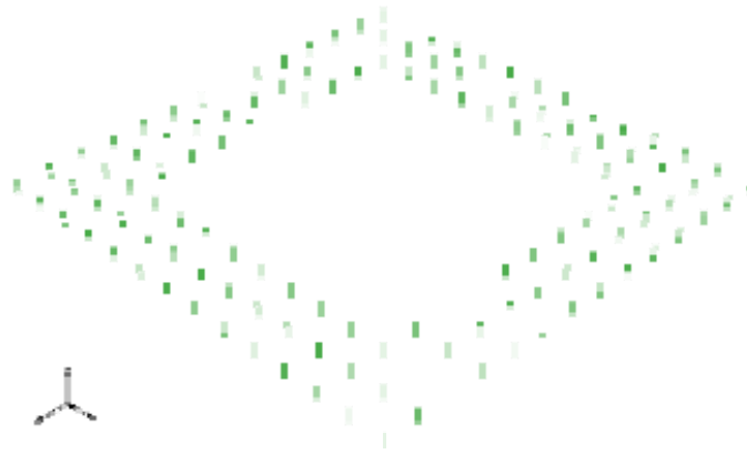
Figure 24 Solder Interconnection Layout Modeled Using Timoshenko Beam elements.
