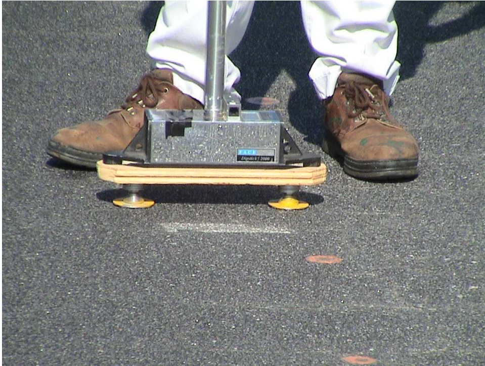
Figure 3.17 DIPSTICK Profile Measurement at the Test Track.
