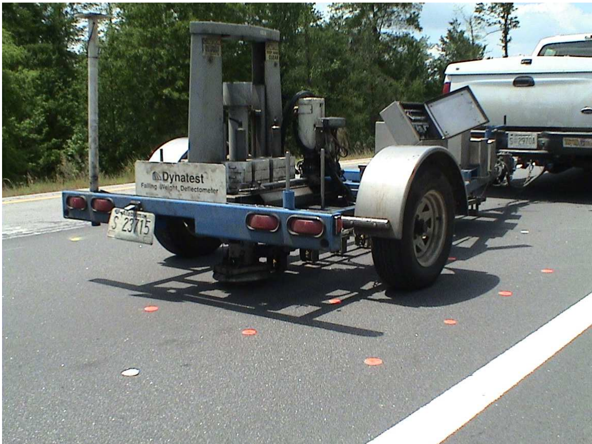
Figure 3.16 FWD Testing on the Structural Study Sections
