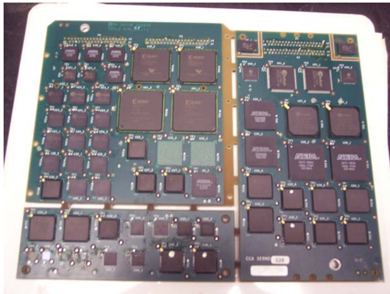
Figure 3.5 Front Side of Test Boards CCA 028-036
