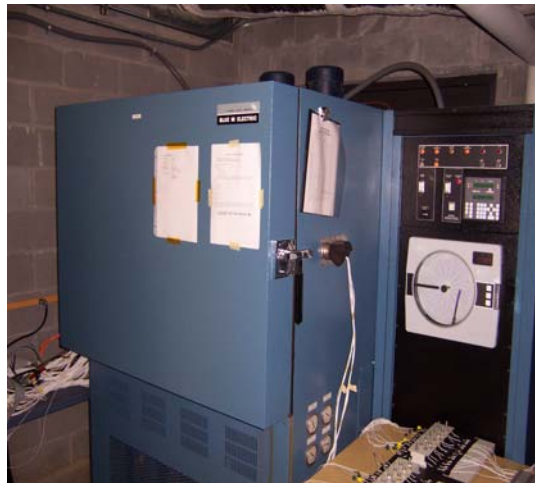
Figure 3.11: Thermal Chamber used for TC2 Temperature Profile
