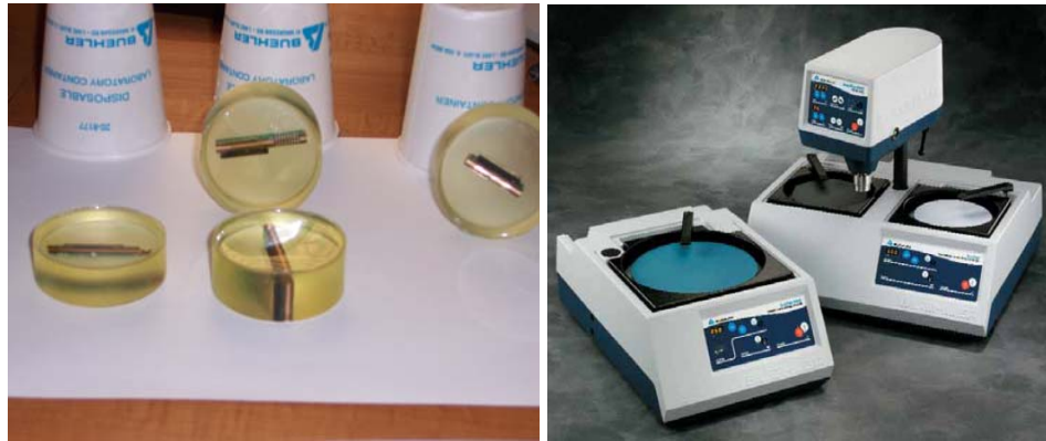
Figure 3.27: Cross-Sectioning Samples and Polisher
