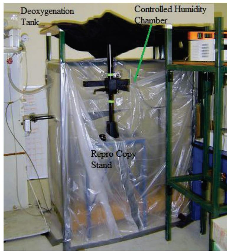
Figure 4.11. Image of SLIF Uni-strut optics bench with the constant humidity enclosure attached.
