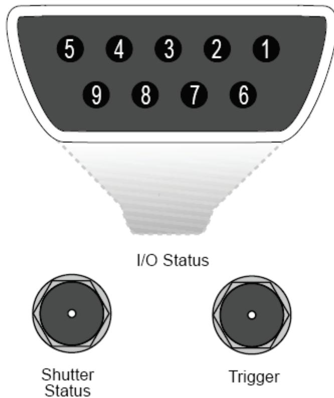
Figure A.1. Diagram of Photometrics 300 CCD camera controller outputs and inputs.
