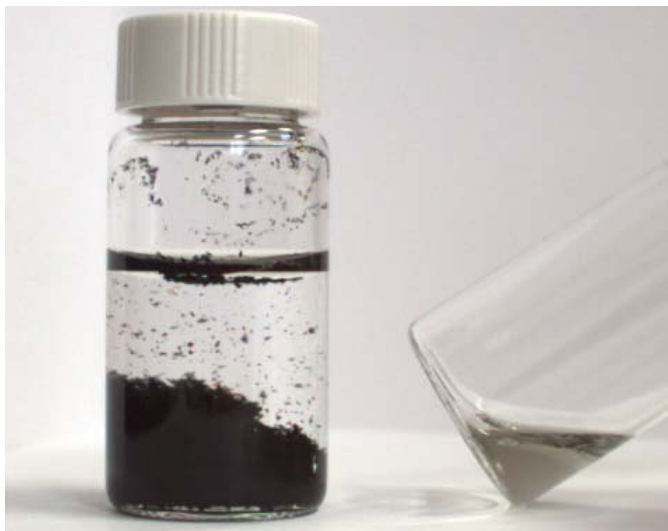
Figure 126: Image of (left) SWNT 183.6 after aggressive tip sonication in water for 30 min. pulsed at 5 s on 1 s off and (right) dilute aqueous solution of lyophilized 6 h oxidized SWNT 183.6 re-dispersed in water by bath sonication.
