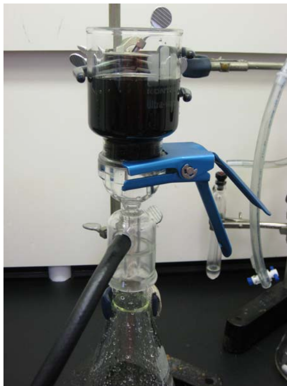
Figure 36: Typical vacuum filtration apparatus used in this research.
