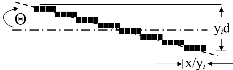
Figure 16: A rod divided into y_i submolecules having x/y_i segments per submolecule and tilted at angle \Theta to the director. The term y_i d represents the height with respect to the director with units of lattice cell number. Reproduced from Beris and Edwards (1994), Cifferi (1994), & Wang and Zhou (2004) [171, 174, 175].
