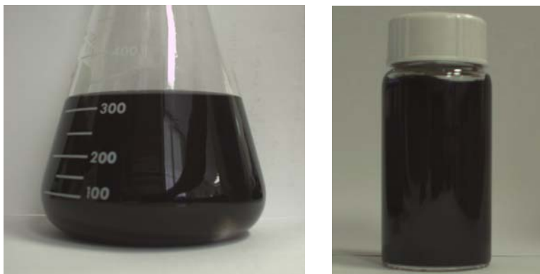
Figure 38: Qualitative proof of successful oxidation. (left) The lack of phase separation in absence of stirring is indication of a stable colloidal suspension. (right) Final aqueous dispersion of neutral, acid oxidized SWNTs. The sample shows excellent dispersion after washing.
