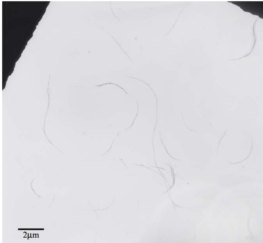
Figure 90: TEM image of the SWNT-UPR dispersion (0.050% vol.) after acetone washing. A mixture of bundled SWNT fibers ranging in lengths and diameters can be seen.
