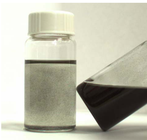
Figure 60: Image of (left) lyophilized 6h oxidized SWNT 183.6 in UPR and (right) a SWNT 183.6 Pure dispersion after the same mixing time. Both samples are at 0.005% vol. loading.
