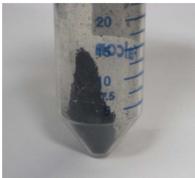
Figure 63: A 6h oxidized sample as it appeared from the freeze dryer. The sample mass was 15 mg before treatment.
