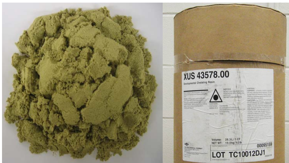
Figure 3-1. The parent chelating resin XUS 3N (1 ft 3 ) received from Dow Chemical.
