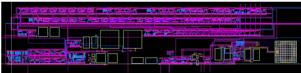
Figure 9.1: Phase locked loop RFIC layout in Cadence environment (2.4mm x 1mm)
