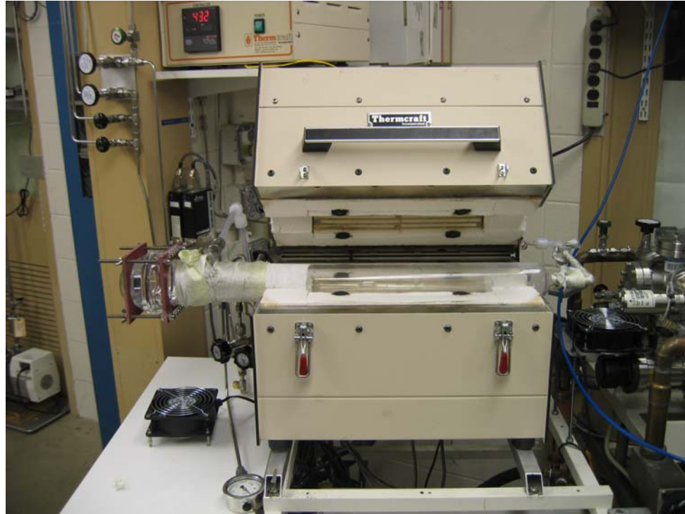
Figure 3.1.3 Furnaces designated for alumina enhanced oxidation.
