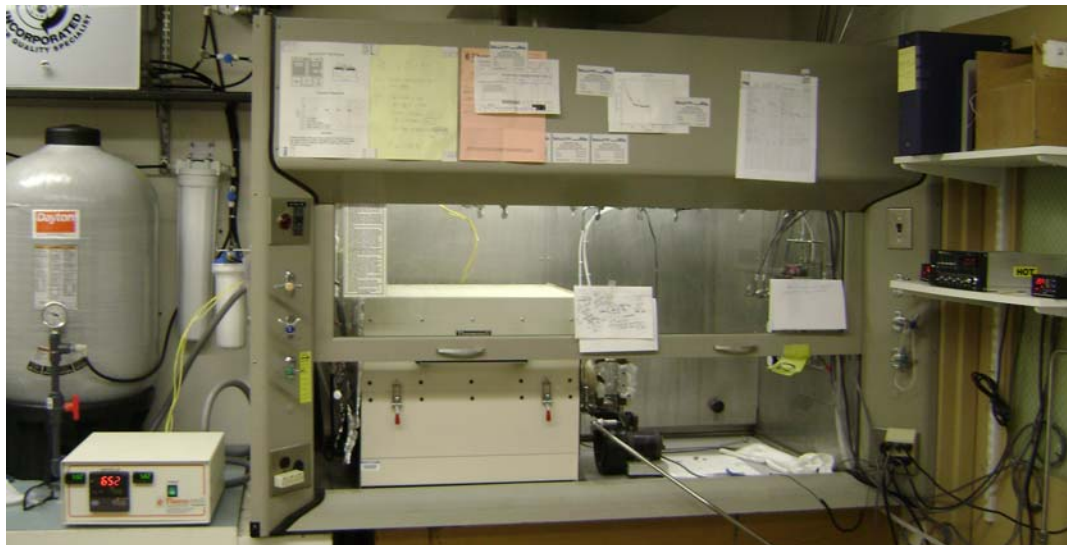
Figure 3.1.2 Furnace used for standard oxidation and few annealing process.
