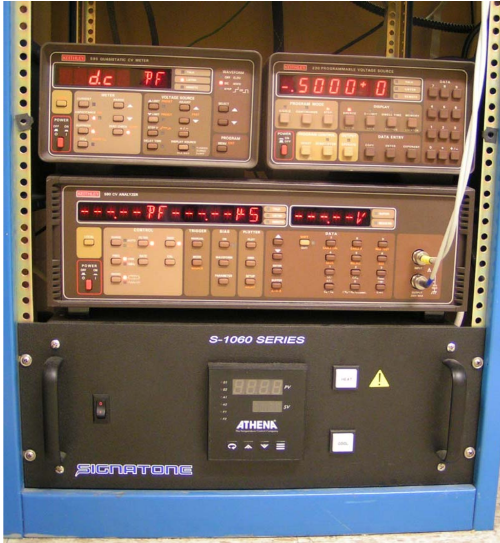
Figure 3.7.2 Keithley CV analyzers and temperature controller for C-V measurement.
