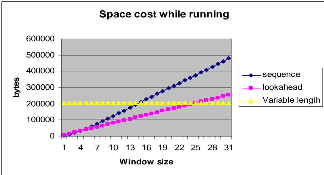
Figure 5.8. Space cost while running of the structures holding the normal pattern DB entries of sequence, lookahead and Variable-Length with Overlap-Relationship Profile Methods.
