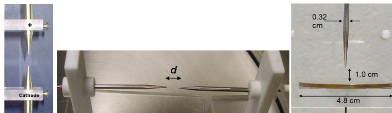
Figure 29. Electrode geometries: (a) point-to-point electrode (b) point-to-point electrode and (c) point-to-plane electrode (Plane electrode always grounded) (All point electrodes have a tip radius = 0.5 mm)
