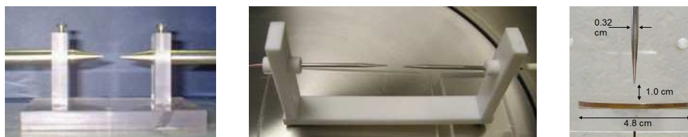
Figure 26. Electrode geometries used in current studies
