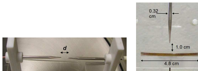
Figure 51. Electrode geometries: (a) point-to-point electrode and (b) point-to-plane electrode (Plane electrode always grounded) (All point electrodes have a tip radius = 0.5 mm)
