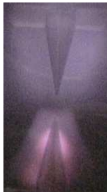
Figure 41. Optical image of the glow discharge during a breakdown event at 20 kHz at 1.4 Torr, point-to-point electrode. (Anode on top, images captured at 30 fps).
