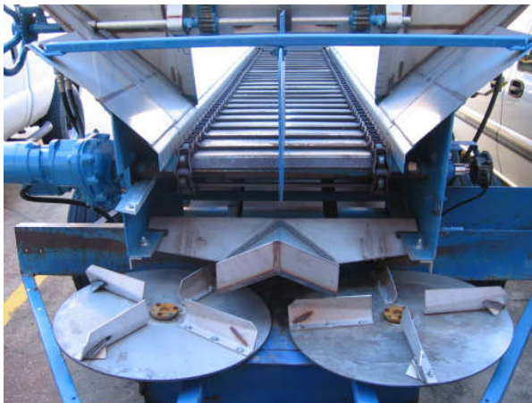
Figure A.3. Litter spreader rear gate, conveyor chain, flow divider and spinners.
