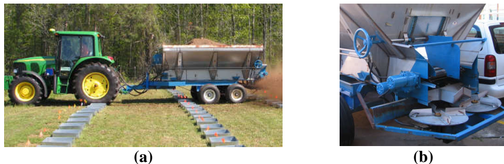
Figure 3.1. Tractor, litter spreader, and illustration of collection pan matrix utilized during testing (a) and rearview image of spreader showing spinner-discs (b).
