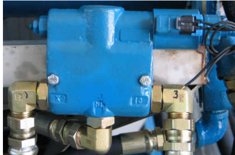
Figure C.1. Brand proportional valve used for spinner and conveyor control.
