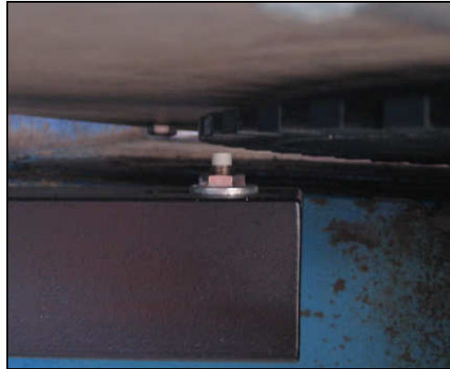
Figure E.1. Sensors to monitor spinner speeds.
