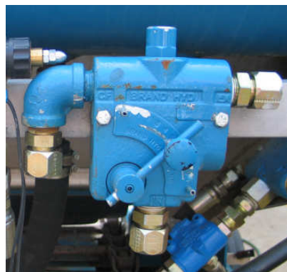
Figure C.2. Brand manual valve used for spinner control.
