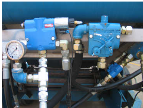
Figure 3.2. Illustration of the two different flow control valves used during testing with the proportional valve shown on the left and manual valve on the right.
