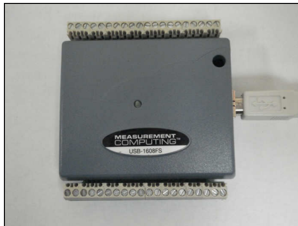
Figure E.4. USB data logger for pressure data.
