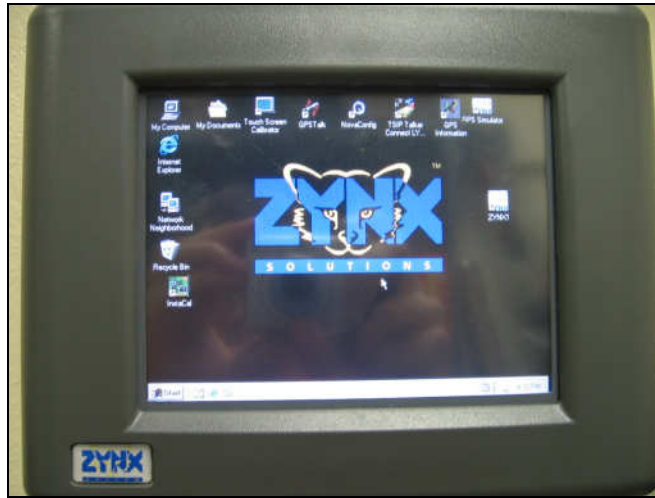
Figure D.2. X15 console used for collecting speed and pressure data.
