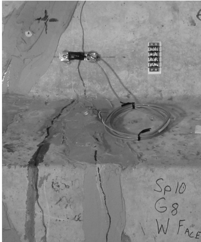
Figure 4-15: Crack Opening Device Installed on Girder
