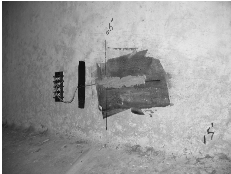
Figure 4-2: Strain Gage After Being Coated with RTV for Moisture Protection
