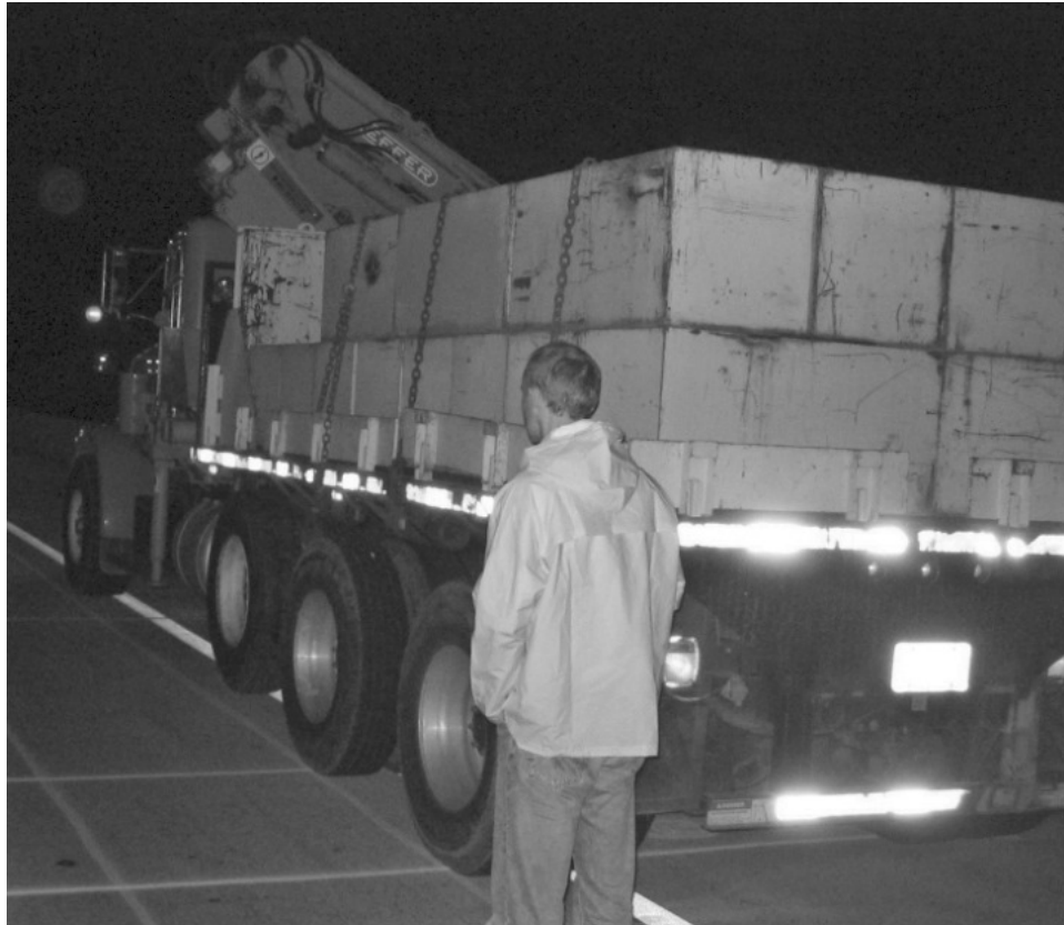
Figure 5-6: Load truck aligned with driver's side rear tires on lane line
