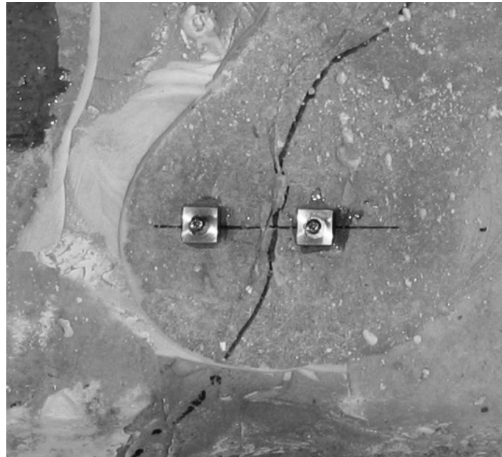
Figure 4-14: Anchor Blocks for COD
