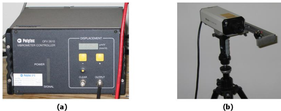
Figure 4.11: Optical Measurement System: (a) Vibrometer Controller, (b) Laser Unit
