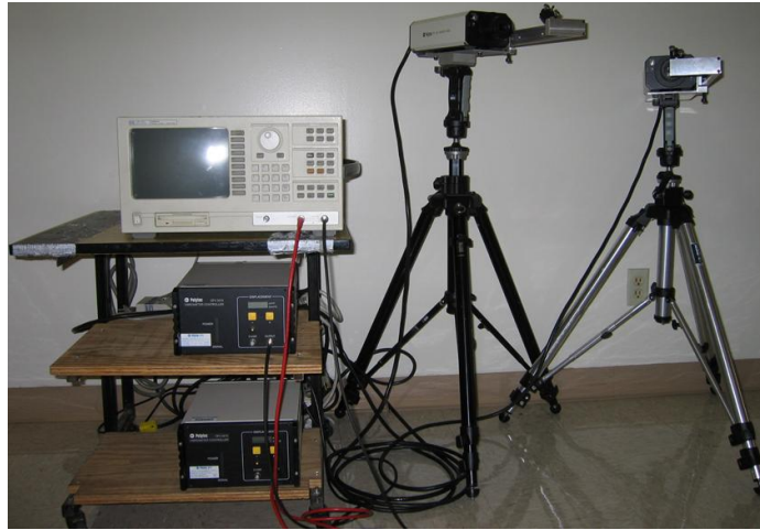
Figure 4.6: Photograph of the Optical Measurement System (two laser units, two controllers, and a signal analyzer)
