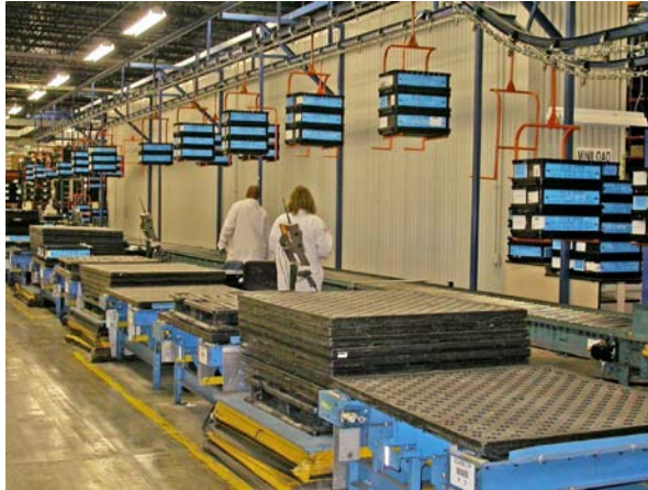
Figure 4.9 Mini-Load AS/RS Accumulation Stands
