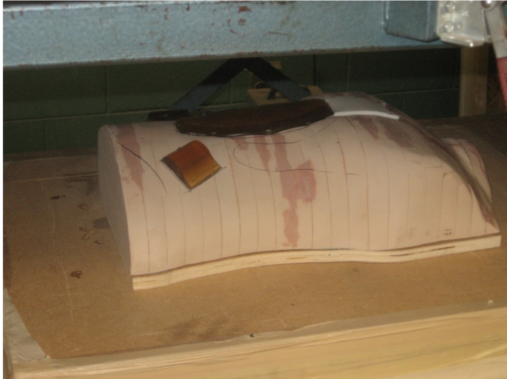
Figure 61. Preparation of the positive mold
