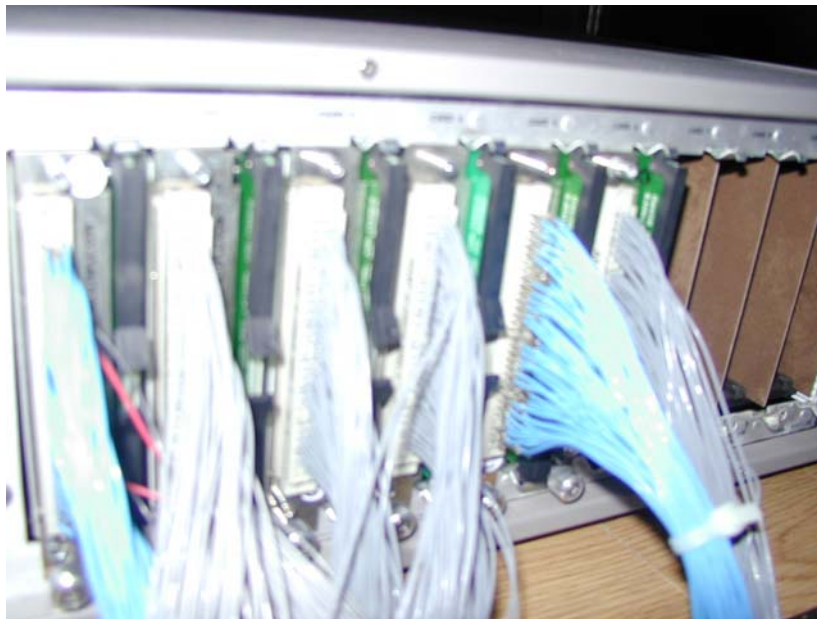
Figure 16 - Multiplexer Cards with Connector Soldering Lugs [19]
