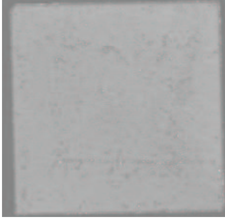
Figure 3.34. C-SAM for assembly with Si (Ti/Au) after 500 thermal shock cycles.
