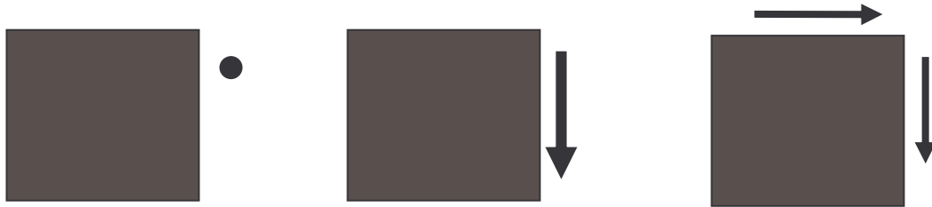
Figure 1.6. Dot, line and “L” shape underfill dispense pattern
