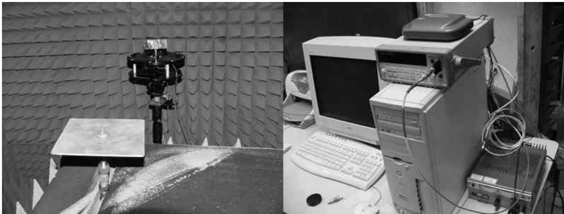
Figure 12 —Pattern measurement equipment, left: transmitting antenna and receiving antenna connected to turntable in anechoic chamber, right: DC power supply, platform controller, digital multimeter, and computer, not shown: power amplifier and RF detector
