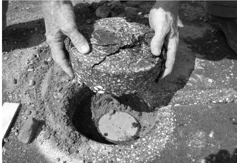
Figure 6 —Source antenna covered by the asphalt plug
