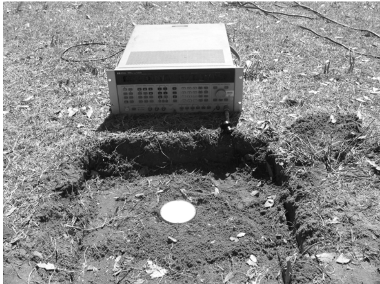
Figure 3 —Buried antenna (uncovered) and signal generator
