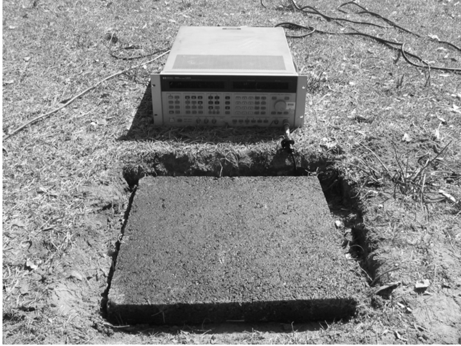
Figure 4 —Buried antenna (covered by asphalt slab) and signal generator
