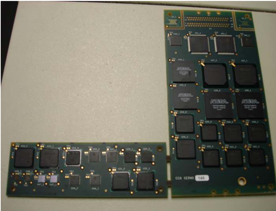
Figure 3.8 Back Side of test board CCA 145-154 (TC4: -20C to 60C).
