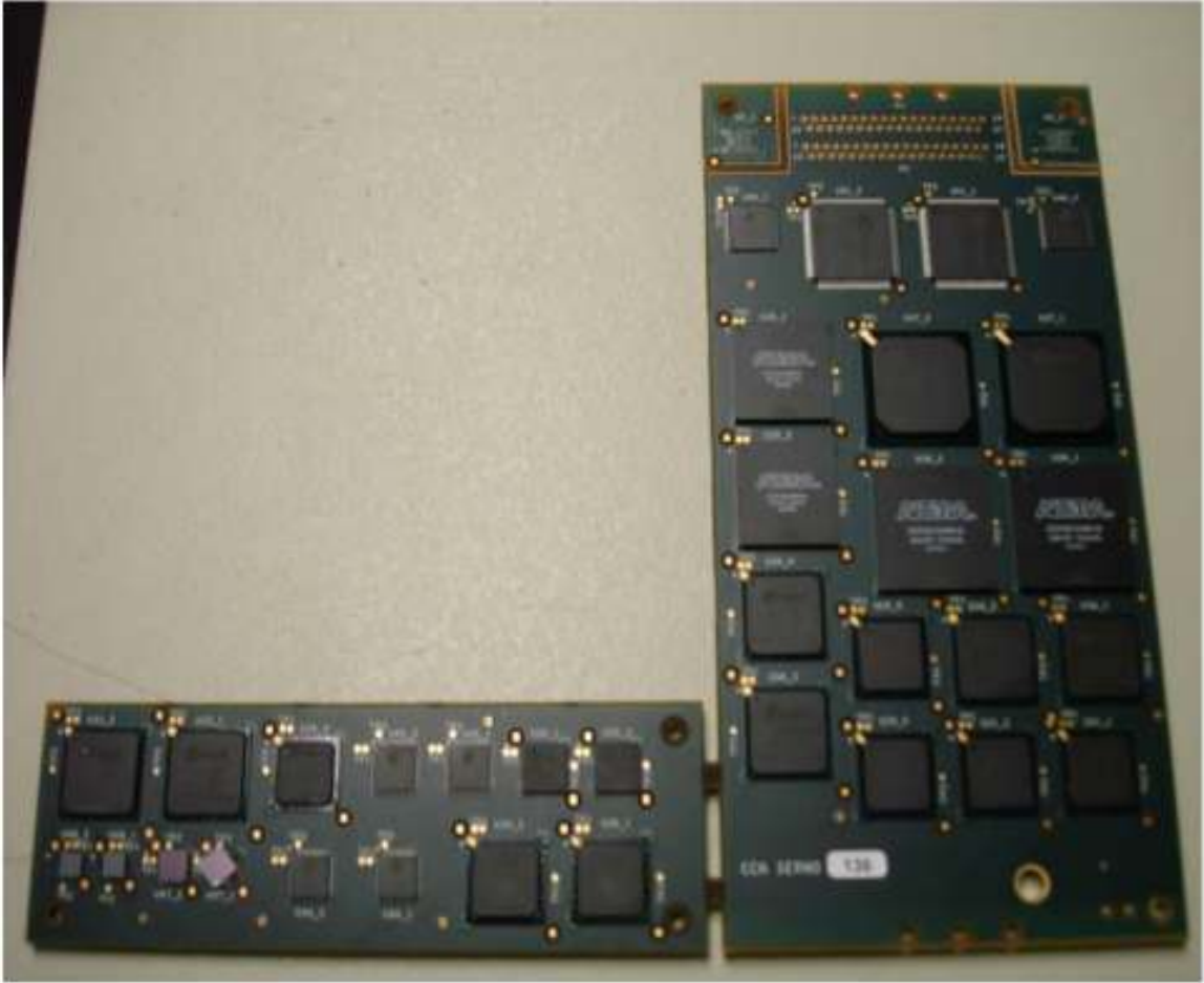
Figure 3.6 Back Side of Test Board CCA 136-144 (TC3: 3C to 100C).
