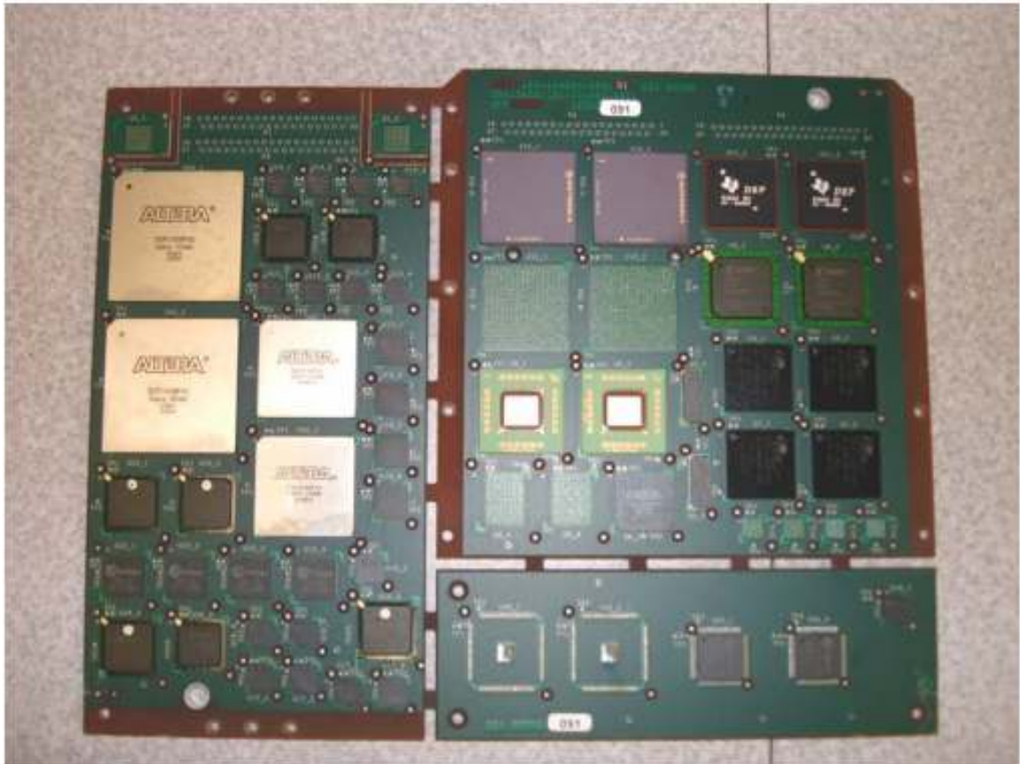
Figure 3.3 Front Side of test board CCA 091-099 (TC2: -55C to 125C).
